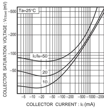
Fig.5 Collector-emitter saturation voltage vs. collector current (I)
