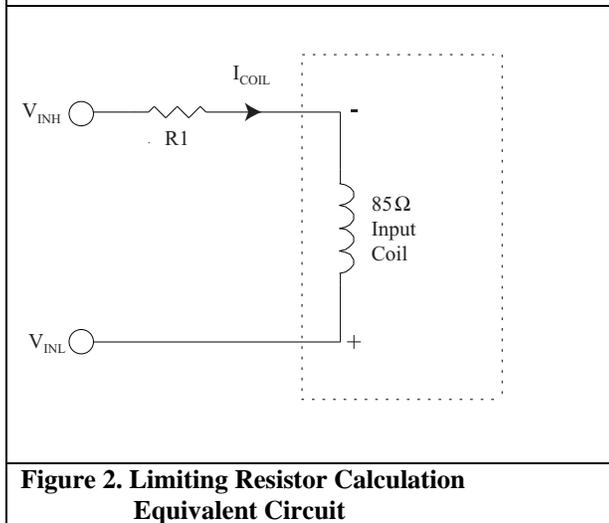
**Figure 2. Limiting Resistor Calculation Equivalent Circuit**
