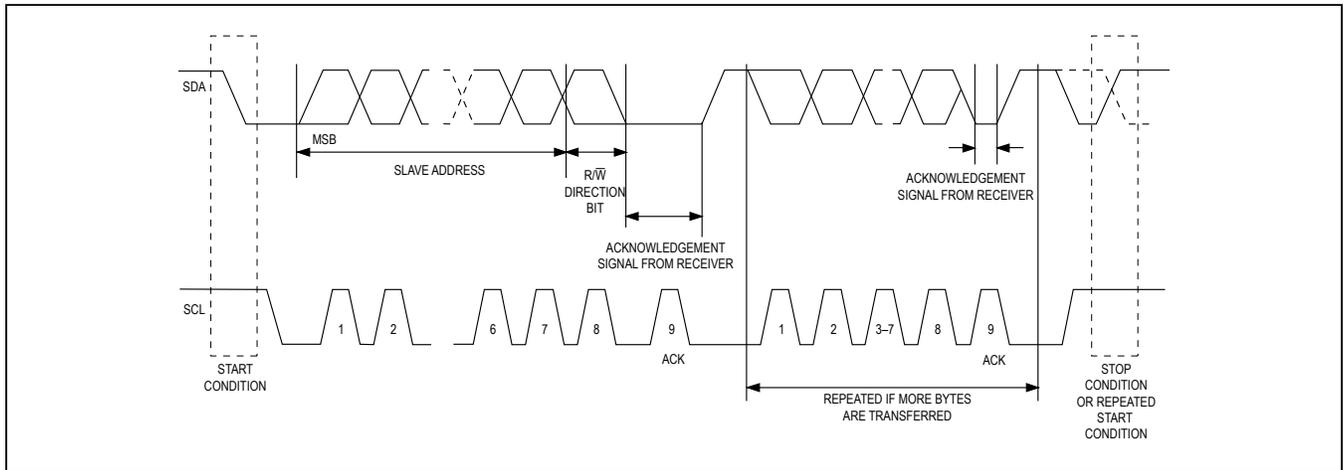
Figure 3. I<sup>2</sup>C Data Transfer Protocol
