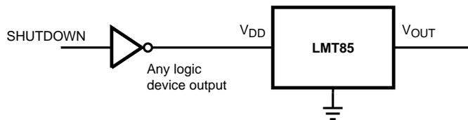
Figure 14. Simple Shutdown Connection of the LMT85-Q1
