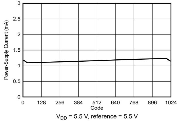
Figure 7-47. Power-Supply Current vs Digital Input Code
