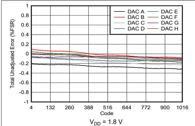
Figure 7-14. Total Unadjusted Error vs Digital Input Code
