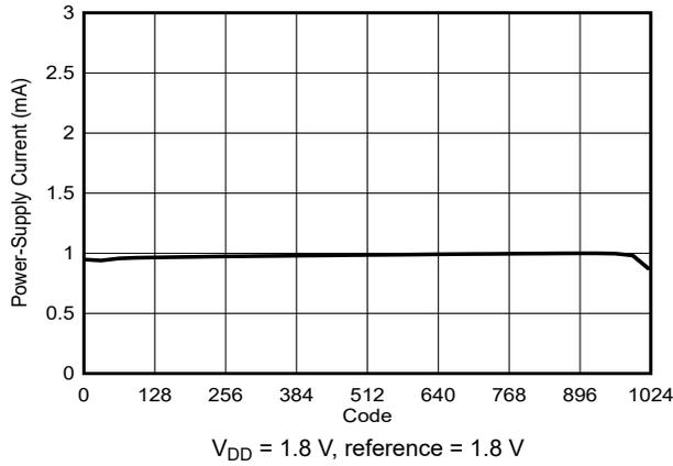
Figure 7-46. Power-Supply Current vs Digital Input Code
