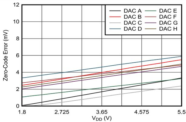
Figure 7-22. Zero-Code Error vs Supply Voltage
