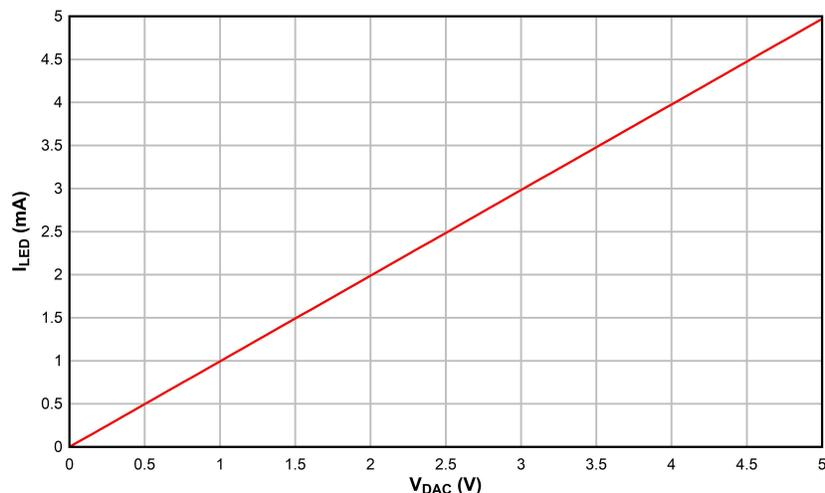
**Figure 9-2. DC Transfer Characteristics of LED Biasing Circuit**
