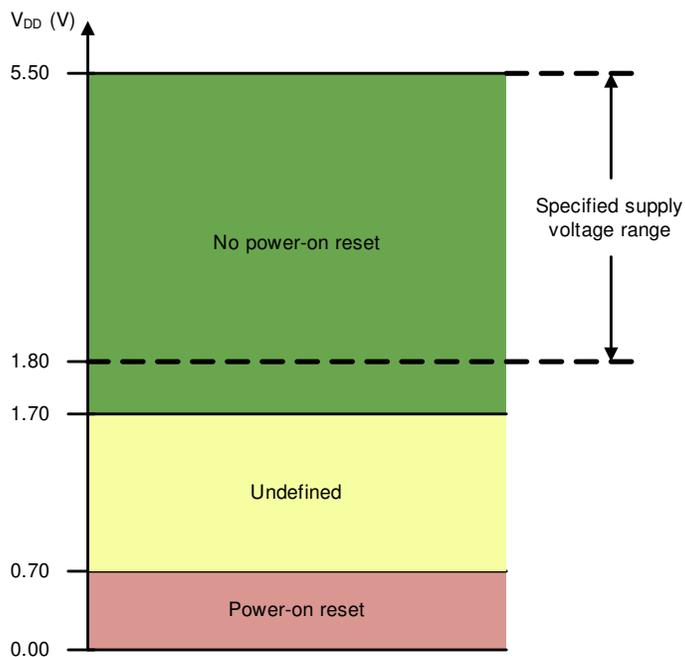
Figure 8-2. Threshold Levels for  $V_{DD}$  POR Circuit
