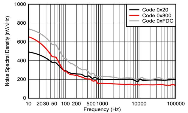
**Figure 7-45. Noise Spectral Density**
