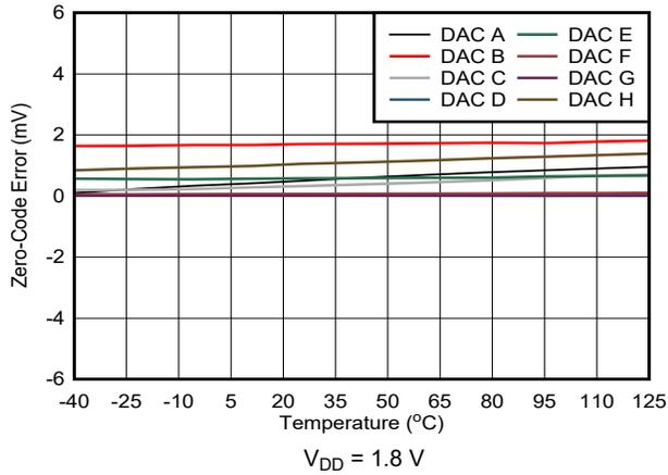
Figure 7-20. Zero-Code Error vs Temperature
