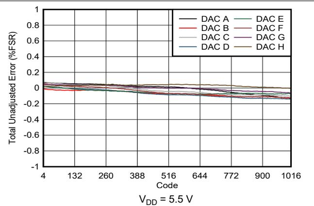
Figure 7-15. Total Unadjusted Error vs Digital Input Code
