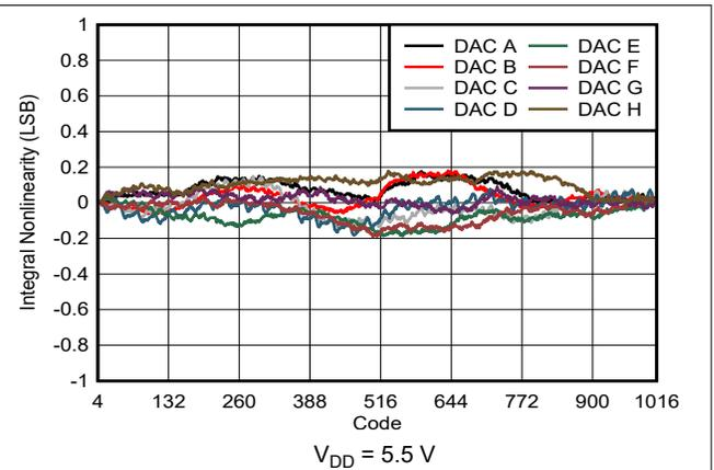
Figure 7-3. Integral Nonlinearity vs Digital Input Code
