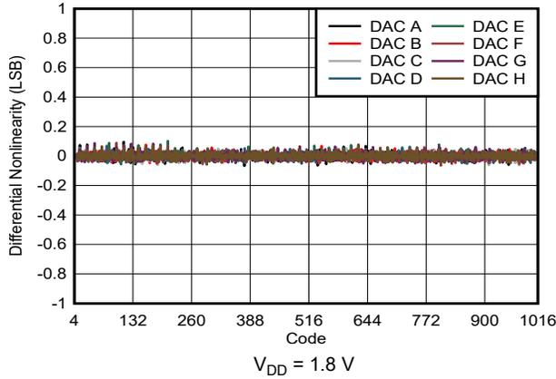
**Figure 7-8. Differential Nonlinearity vs Digital Input Code**
