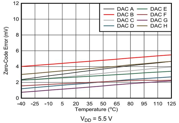
Figure 7-21. Zero-Code Error vs Temperature
