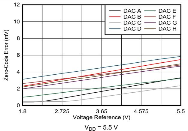
Figure 7-23. Zero-Code Error vs Voltage Reference
