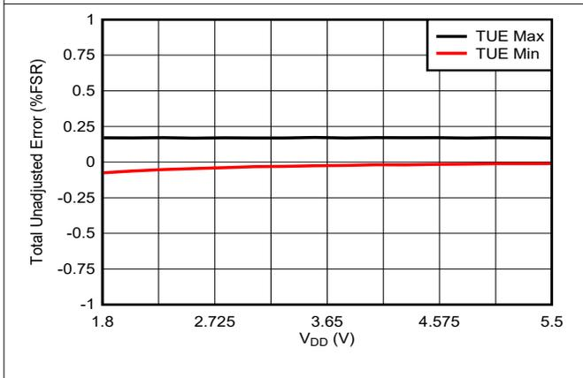
Figure 7-18. Total Unadjusted Error vs Supply Voltage
