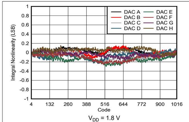
Figure 7-2. Integral Nonlinearity vs Digital Input Code
