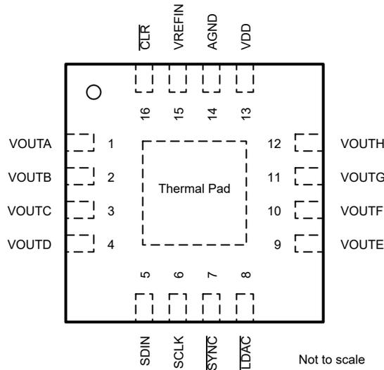
**Figure 6-1. RTE (16-Pin WQFN) Package, Top View**
