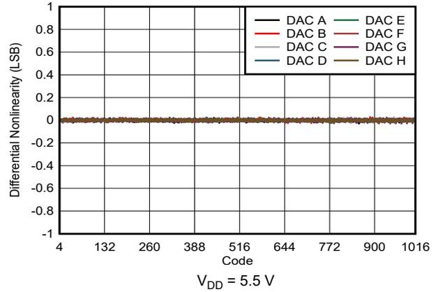
**Figure 7-9. Differential Nonlinearity vs Digital Input Code**
