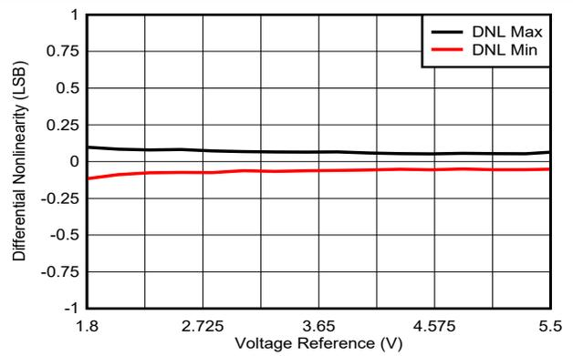
**Figure 7-13. Differential Nonlinearity vs Voltage Reference**
