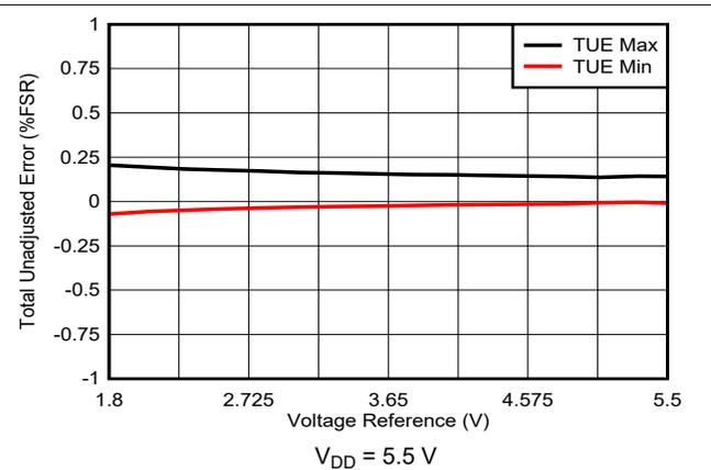
Figure 7-19. Total Unadjusted Error vs Voltage Reference
