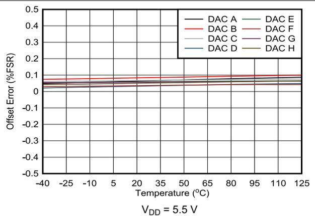
Figure 7-25. Offset Error vs Temperature
