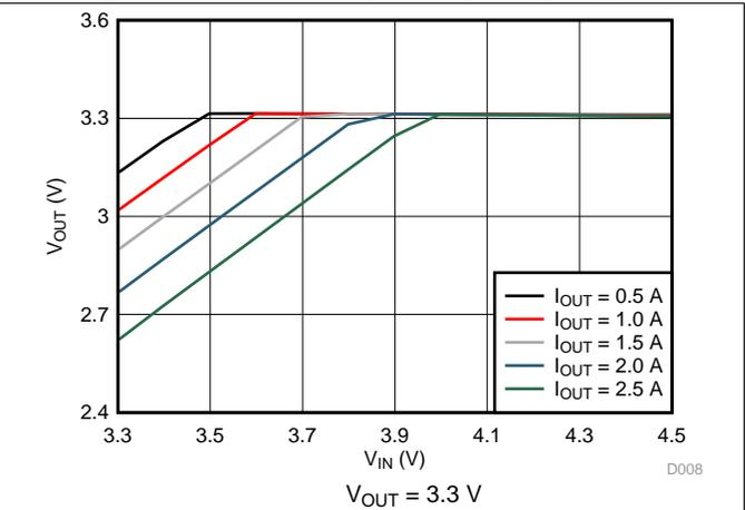
Figure 8. Dropout Curve
