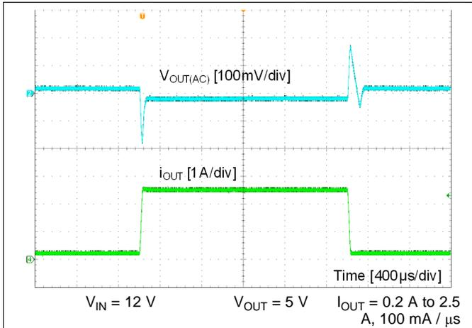
**Figure 29. Load Transient**
