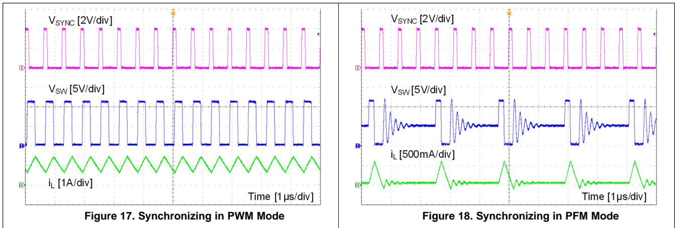
Figure 17. Synchronizing in PWM Mode
