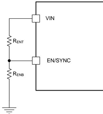
**Figure 15. System UVLO by Enable Divider**
