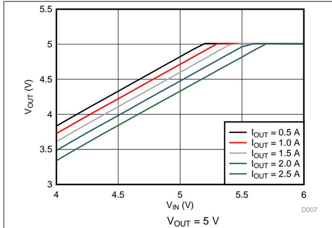
Figure 7. Dropout Curve
