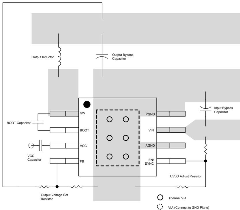
Figure 33. SOIC Layout
