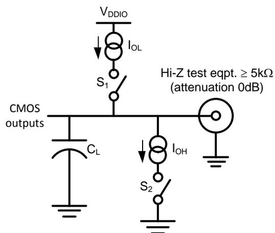
$C_L$  including probe and jig
