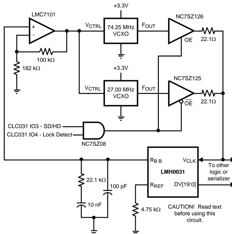
**Figure 8. Using Dual VCXOs for VCLK Example**
