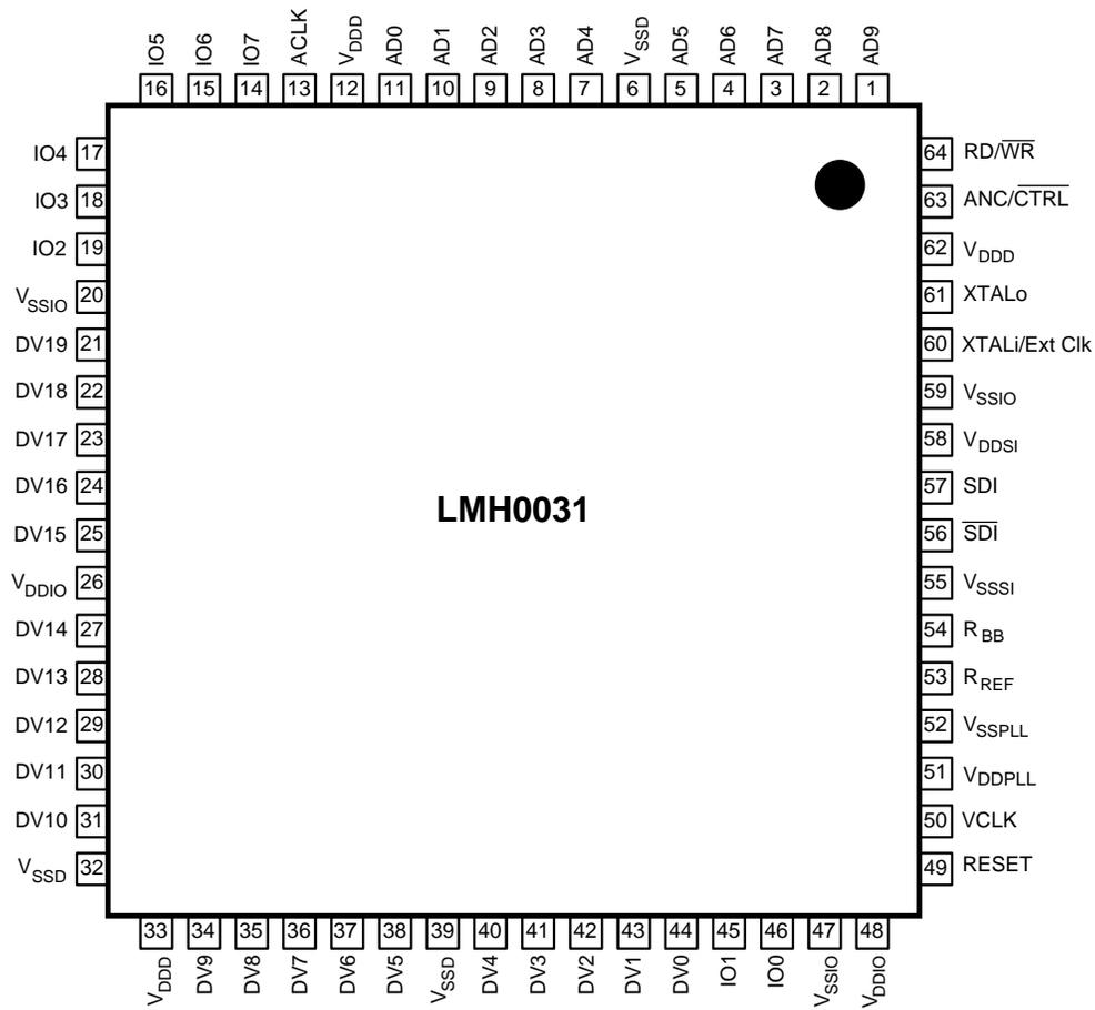
Figure 1. 64-Pin TQFP
