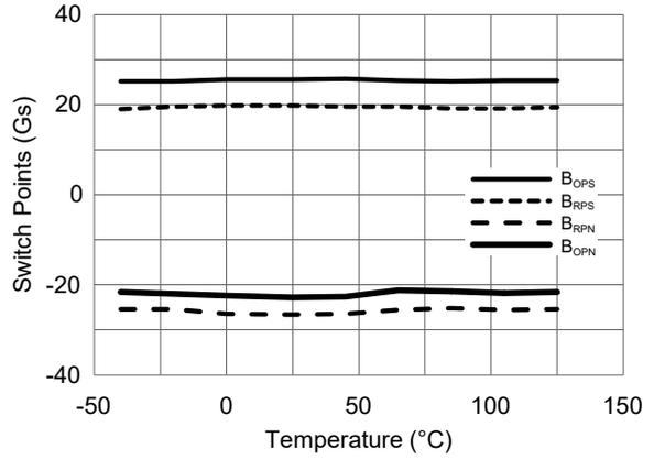
Figure 10. Switch points versus temperature ( $V_{CC} = 3\text{ V}$ )
