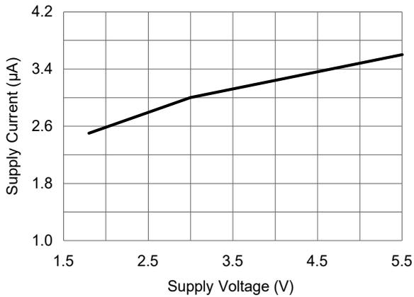
Figure 7. Supply current versus supply voltage ( $T_A=25^\circ\text{C}$ )
