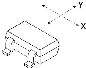
Figure 2. Sensing direction
