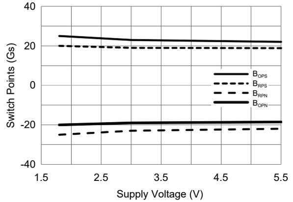
Figure 6. Switch points versus supply voltage ( $T_A=25^\circ\text{C}$ )
