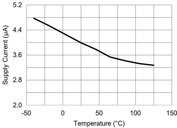
Figure 11. Supply current versus temperature ( $V_{CC} = 3\text{ V}$ )
