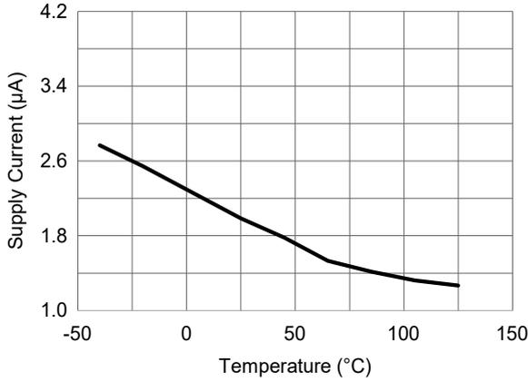
Figure 9. Supply current versus temperature ( $V_{CC} = 3\text{ V}$ )
