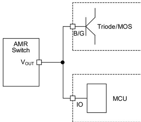
Figure 14. Application diagram for driving power load
