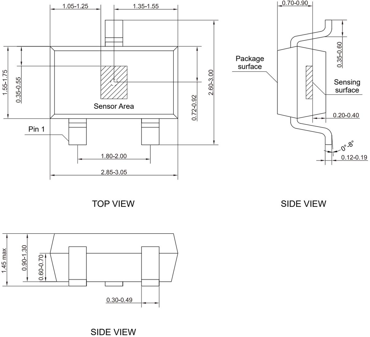
Figure 15. Package outline of SOT23-3 (unit: mm)
