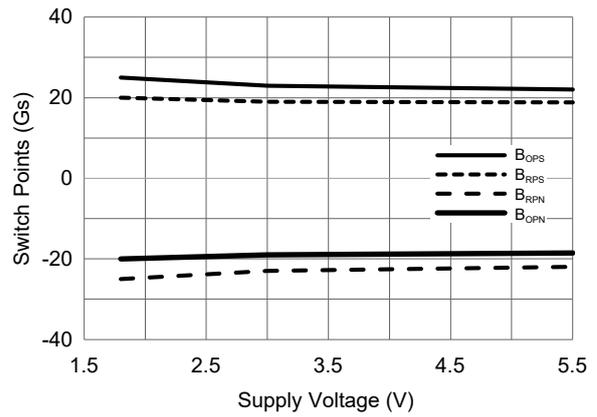
Figure 8. Switch points versus supply voltage ( $T_A=25^\circ\text{C}$ )
