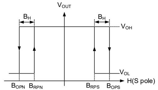
Figure 3. Switching characteristics
