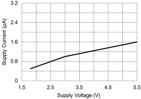
Figure 5. Supply current versus supply voltage ( $T_A=25^\circ\text{C}$ )
