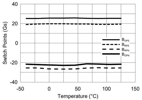
Figure 12. Switch points versus temperature ( $V_{CC} = 3\text{ V}$ )
