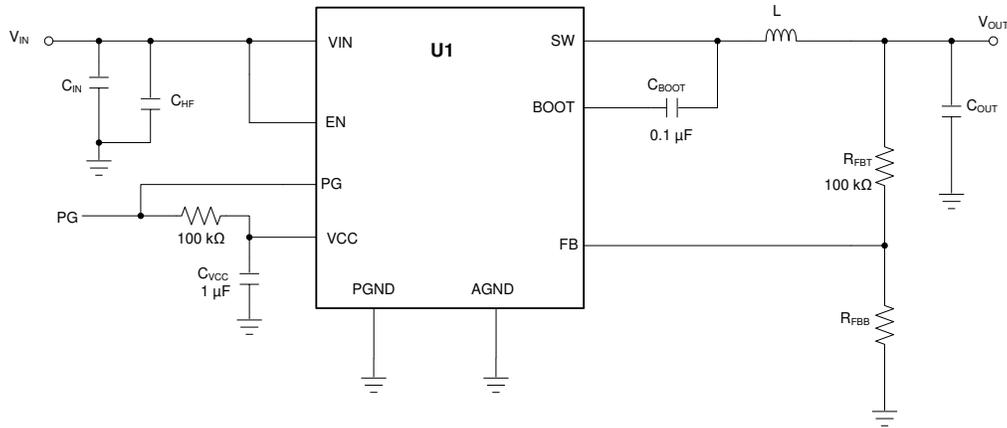
**Figure 9-21. Circuit for Application Curves**
