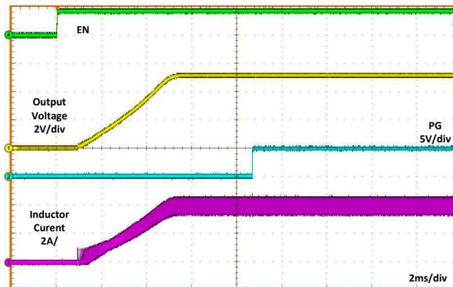
**Figure 8-4. Typical Start-up Behavior  $V_{IN} = 12\text{ V}$ ,  $V_{OUT} = 5\text{ V}$ ,  $I_{OUT} = 4\text{ A}$**
