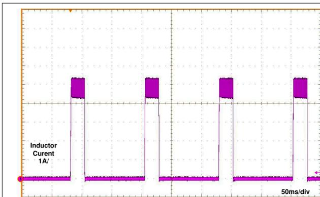
**Figure 8-5. Inductor Current Burst in Short-Circuit Mode**
