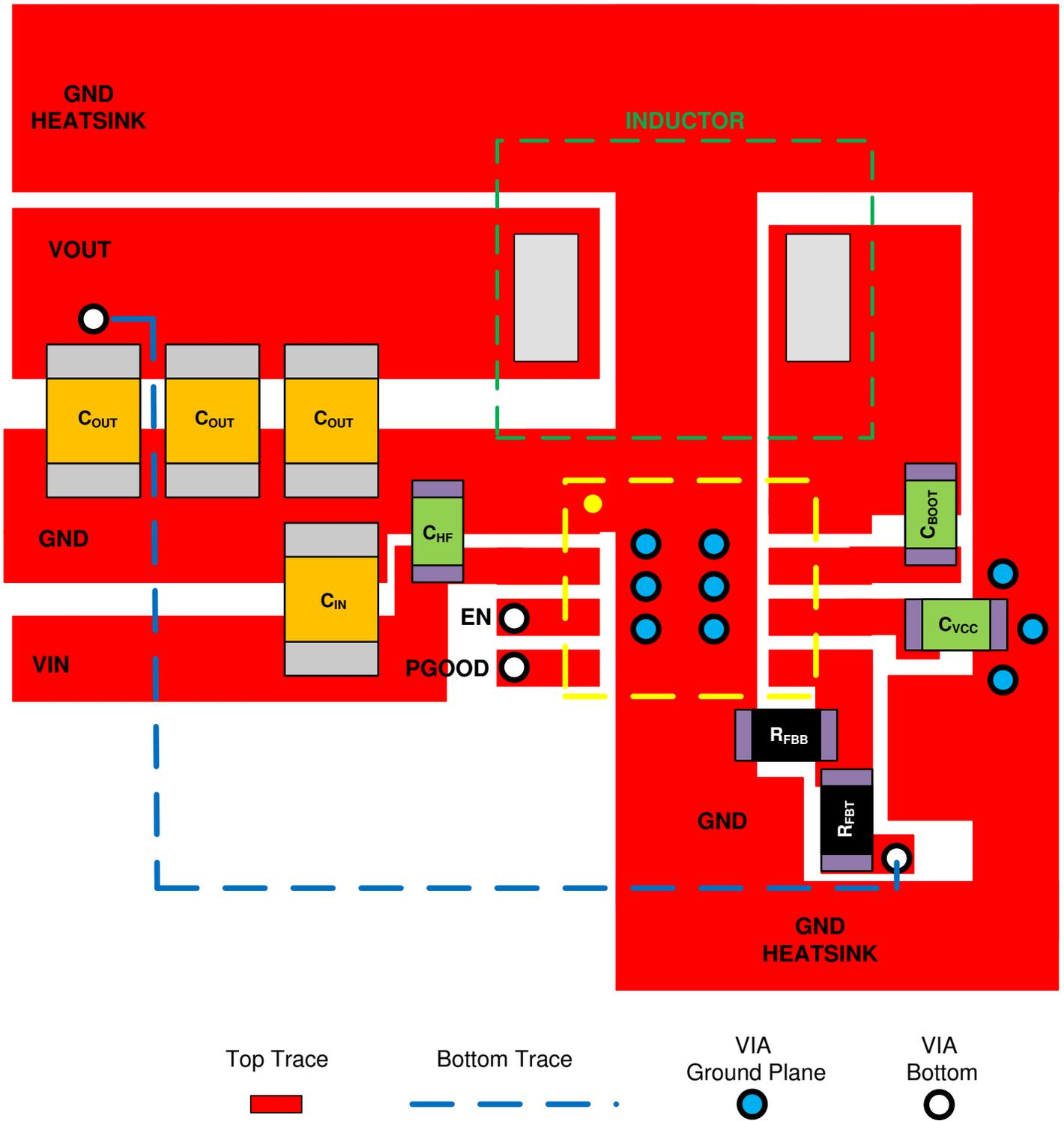
Figure 11-2. Example Layout for HSOIC (DDA) Package
