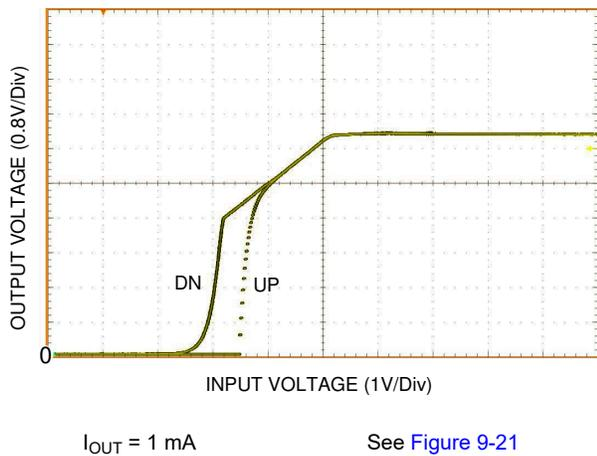
**Figure 7-5. UVLO Thresholds**
