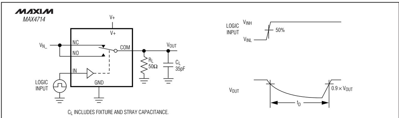
Figure 2. Break-Before-Make Interval
