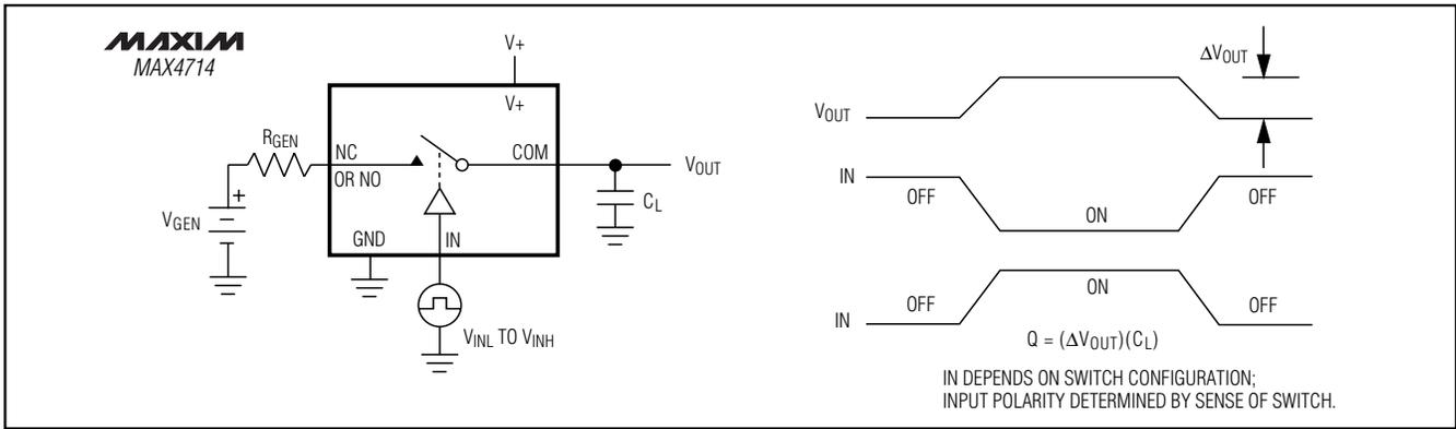
Figure 3. Charge Injection
