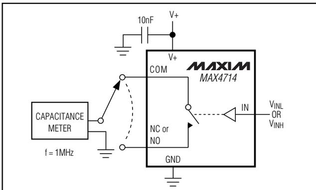
Figure 5. Channel Off/On-Capacitance
