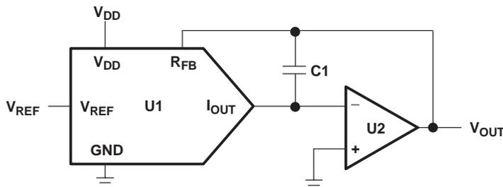
Figure 20. Gain Peaking Prevention Circuit With Compensation Capacitor
