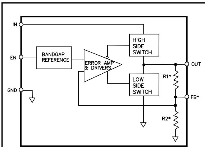
\* R1 and R2 are only in fixed voltage parts. FB pin is only present in adjustable part.
