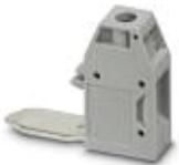
Pick-off terminal block, Connection method: Screw connection, Cross section: 0.5 mm<sup>2</sup> - 10 mm<sup>2</sup>, AWG: 20 - 8, Width: 10.2 mm, Height: 34.7 mm, Color: gray, Mounting type: On base element
