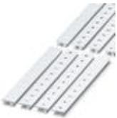
Zack marker strip, Strip, white, labeled, can be labeled with: Plotter, Printed vertically: Consecutive numbers 1 - 10, 11 - 20, etc. up to 991 - 1000, Mounting type: Snap into tall marker groove, for terminal block width: 10.2 mm, Lettering field: 10.15 x 10.5 mm
