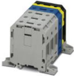
High-current terminal block, Connection method: Screw connection, Number of positions: 5, Cross section: 16 mm<sup>2</sup> - 95 mm<sup>2</sup>, AWG: 4 - 3/0, Width: 101.5 mm, Height: 80 mm, Color: gray/blue/black-yellow, Mounting type: ct screw connection
