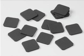
Eccosorb FGM is a thin, flexible, magnetically loaded, silicone absorber. Silicone absorbers have high service temperature capabilities and offer advantages for high power and low outgassing applications. They can be subjected to high altitudes, including space, with no adverse effects.
