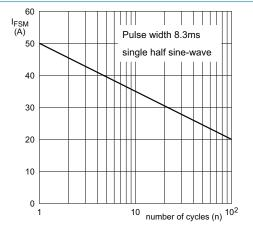
Fig. 5. Pulse rating curve
