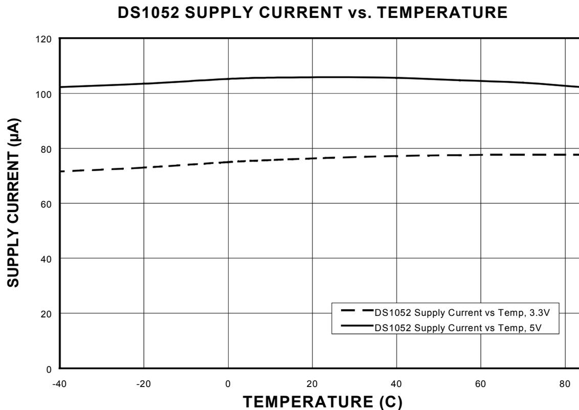
**TYPICAL OPERATING CHARACTERISTICS DS1052** $(V_{CC} = 5.0V; T = +25^{\circ}C, \text{ unless otherwise specified})$
