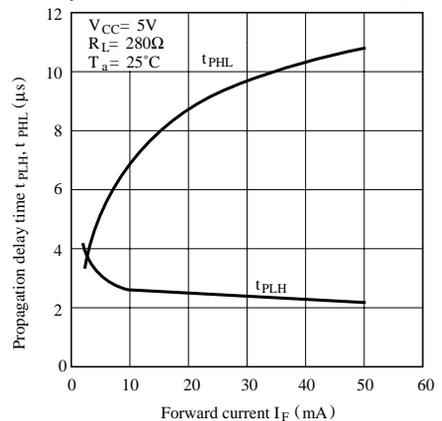
**Fig.10-b Propagation Delay Time vs. Forward Current (GP1A53HR)**
