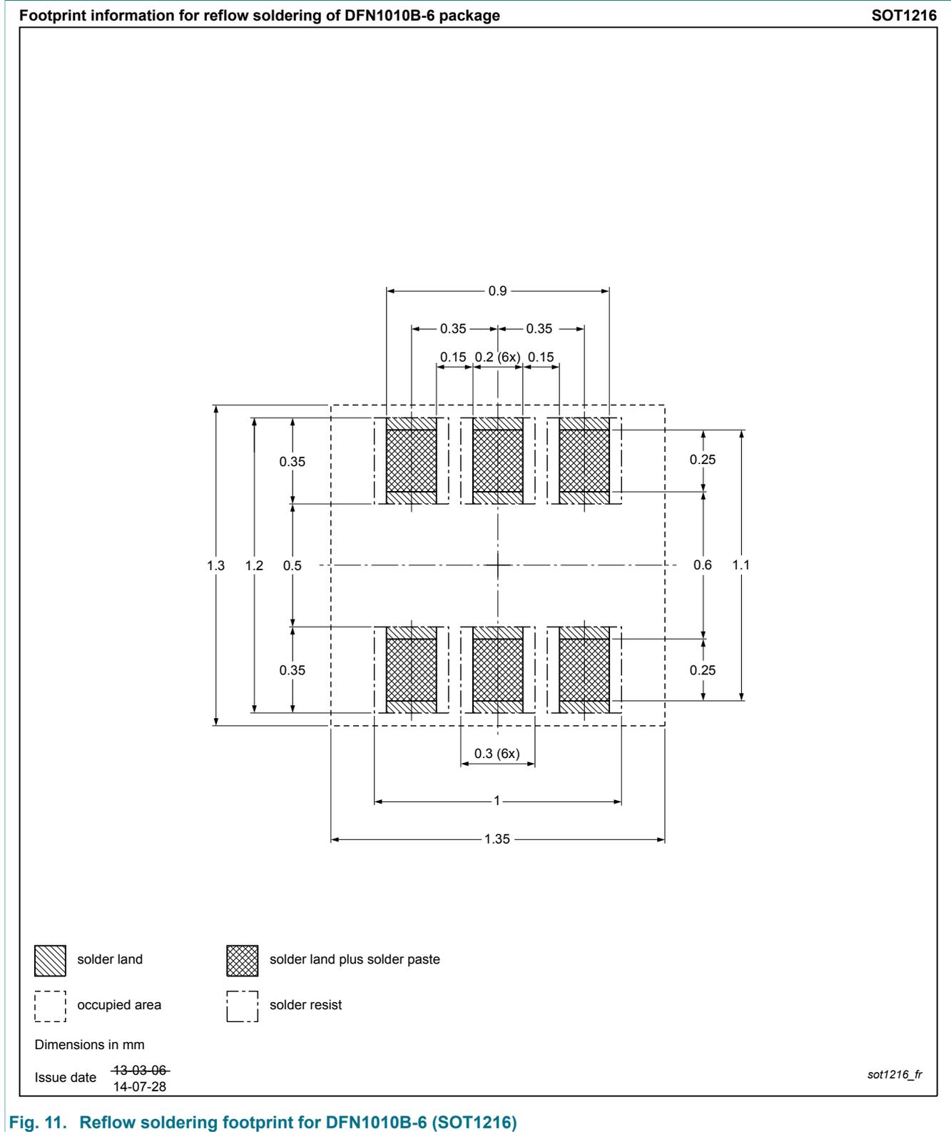
Fig. 11. Reflow soldering footprint for DFN1010B-6 (SOT1216)
