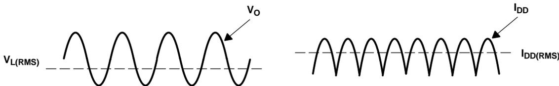
Figure 25. Voltage and Current Waveforms for BTL Amplifiers
