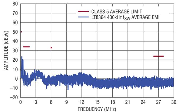
12V INPUT TO 24V OUTPUT AT 1A, f<sub>SW</sub> = 400kHz
