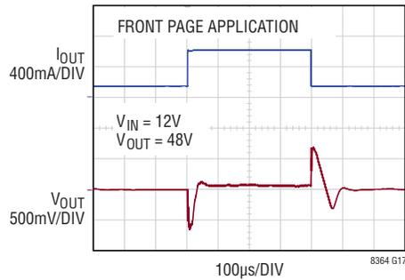
**V<sub>OUT</sub> Transient Response: Load Current Transients from 320mA to 640mA to 320mA**
