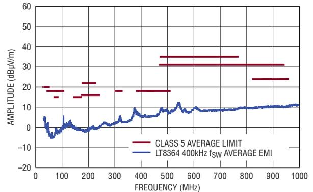
12V INPUT TO 24V OUTPUT AT 1A, f<sub>SW</sub> = 400kHz
