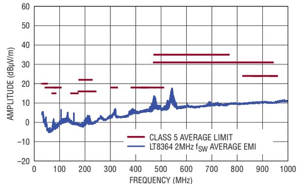
12V INPUT TO 24V OUTPUT AT 1A,  $f_{SW} = 2MHz$
