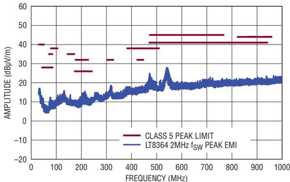
12V INPUT TO 24V OUTPUT AT 1A,  $f_{SW} = 2MHz$
