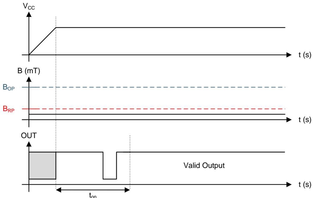
**Figure 14. Case 2: Power On When  $B < B_{RP}$**
