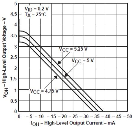
Figure 5-5. High-Level Output Voltage vs High-Level Output Current
