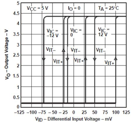
Figure 5-4. Receiver Output Voltage vs Differential Input Voltage
