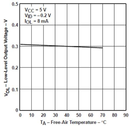
**Figure 5-8. Receiver Low-Level Output Voltage vs Free-Air Temperature**
