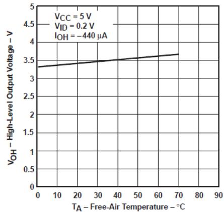
Figure 5-6. High-Level Output Voltage vs Free-Air Temperature
