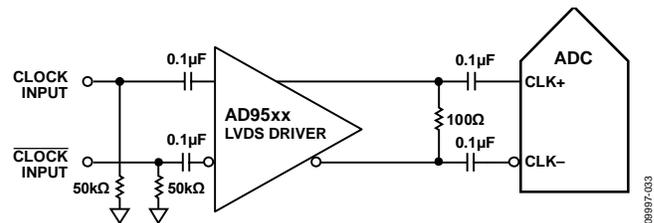
Figure 33. Differential LVDS Sample Clock (Up to 625 MHz)
