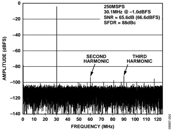
Figure 4. Single-Tone FFT with  $f_{IN} = 30.1$  MHz
