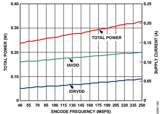
Figure 35. AD6672-250 Power and Current vs. Sample Rate
