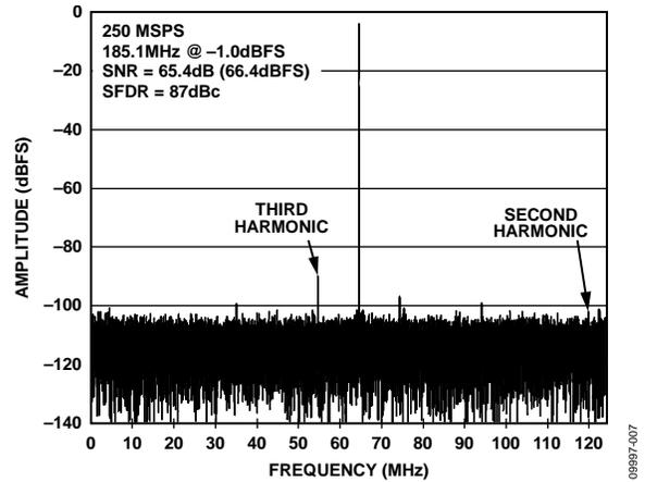
Figure 7. Single-Tone FFT with  $f_{IN} = 185.1$  MHz
