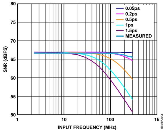
Figure 34. SNR vs. Input Frequency and Jitter
