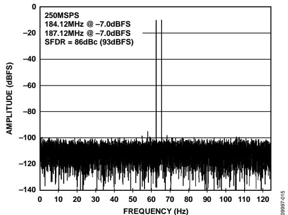
Figure 15. Two-Tone FFT with  $f_{IN1} = 184.12$  MHz,  $f_{IN2} = 187.12$  MHz
