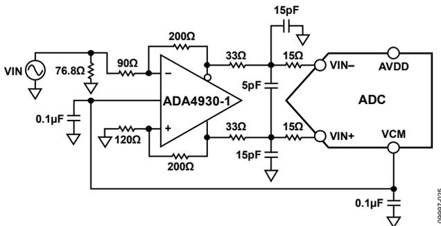
Figure 25. Differential Input Configuration Using the ADA4930-1
