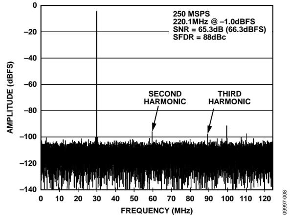
Figure 8. Single-Tone FFT with  $f_{IN} = 220.1$  MHz
