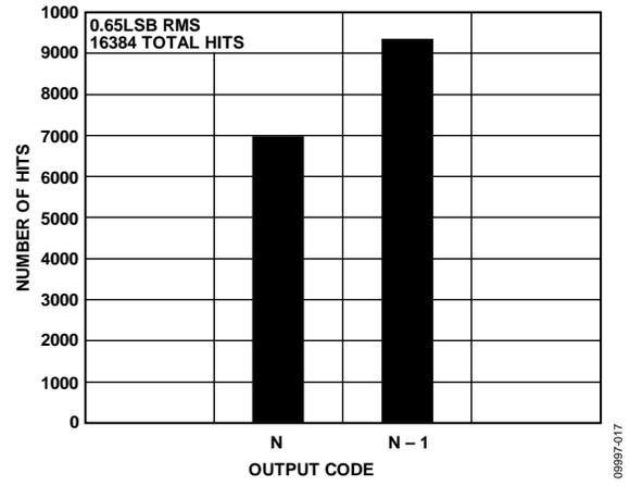
Figure 17. Grounded Input Histogram,  $f_s = 250$  MSPS
