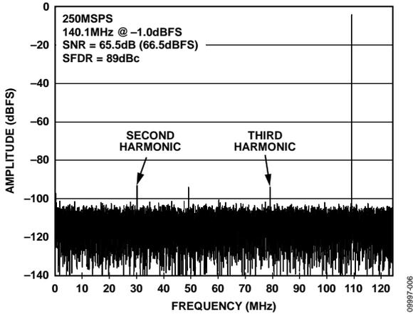
Figure 6. Single-Tone FFT with  $f_{IN} = 140.1$  MHz
