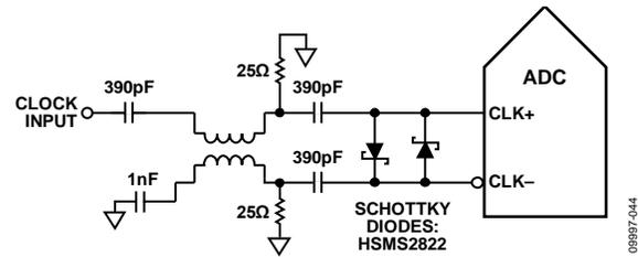
Figure 31. Balun-Coupled Differential Clock (Up to 625 MHz)
