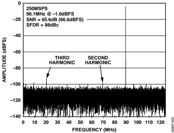
Figure 5. Single-Tone FFT with  $f_{IN} = 90.1$  MHz
