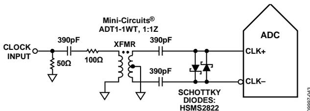
Figure 30. Transformer-Coupled Differential Clock (Up to 250 MHz)
