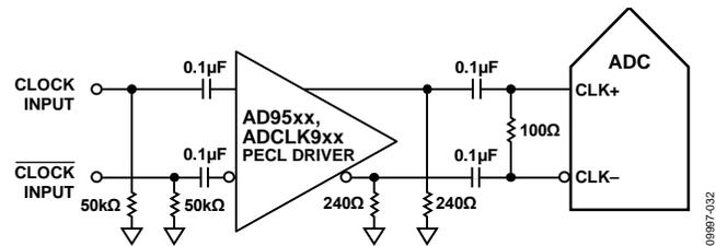
Figure 32. Differential PECL Sample Clock (Up to 625 MHz)
