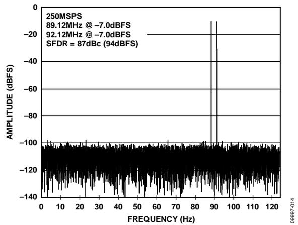
Figure 14. Two-Tone FFT with  $f_{IN1} = 89.12$  MHz,  $f_{IN2} = 92.12$  MHz
