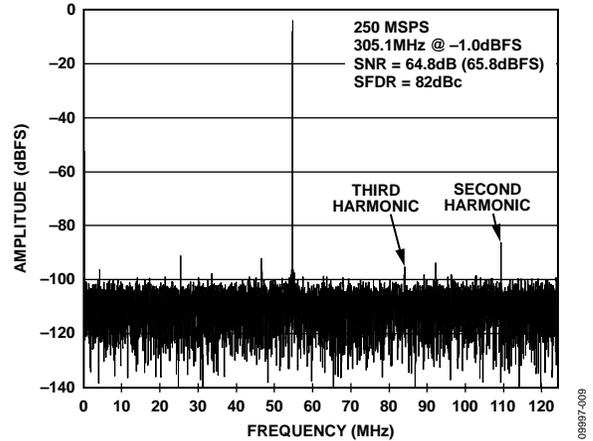
Figure 9. Single-Tone FFT with  $f_{IN} = 305.1$  MHz
