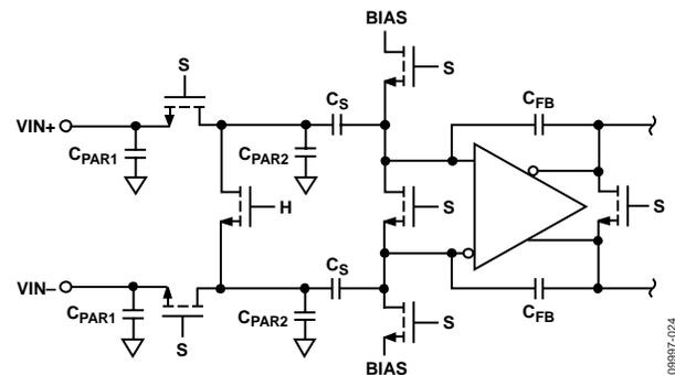
Figure 24. Switched-Capacitor Input
