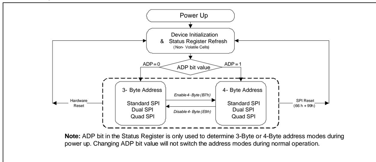
Figure 3. W25Q01JV Serial Flash Memory Operation Diagram
