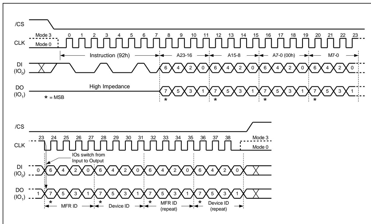
Figure 47. Read Manufacturer / Device ID Dual I/O Instruction
