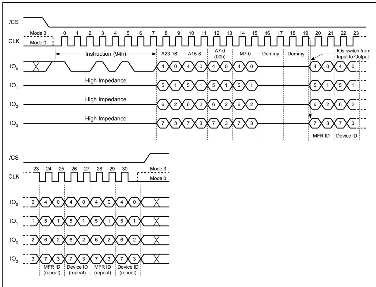
Figure 48. Read Manufacturer / Device ID Quad I/O Instruction
