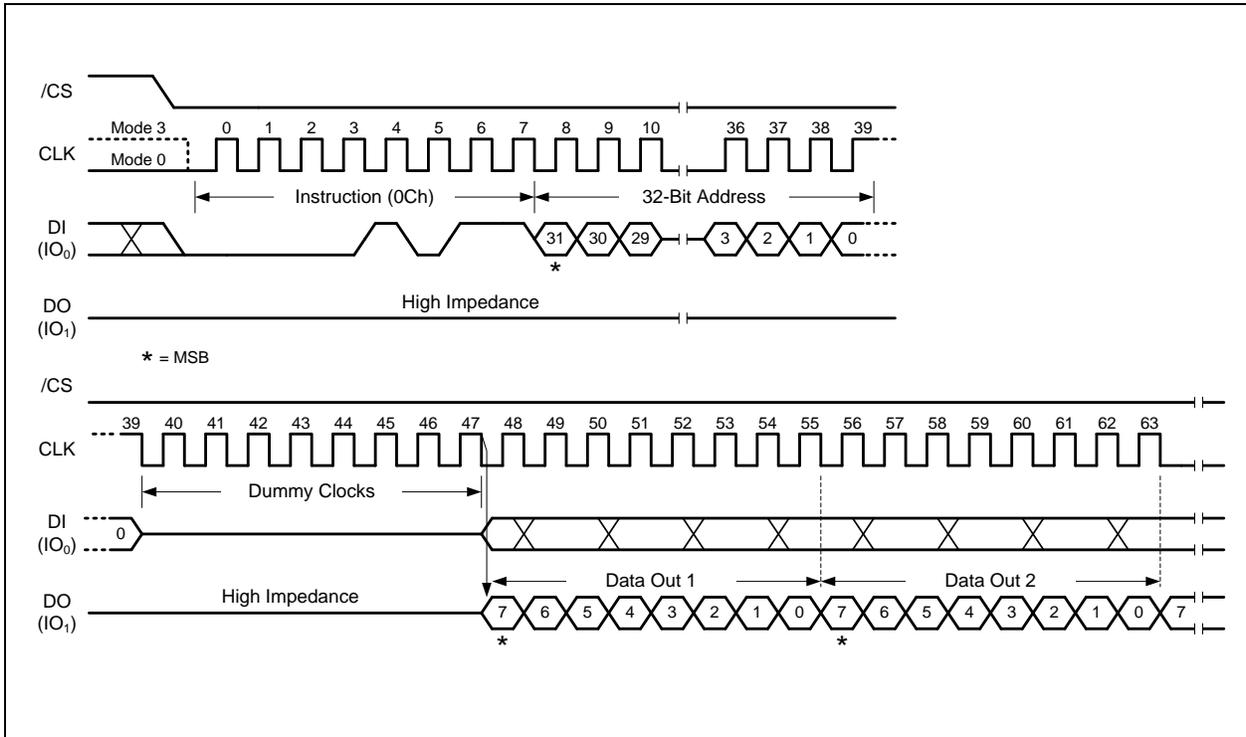
Figure 18. Fast Read with 4-Byte Address Instruction
