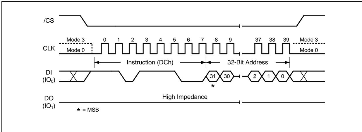
Figure 40. 64KB Block Erase with 4-Byte Address Instruction
