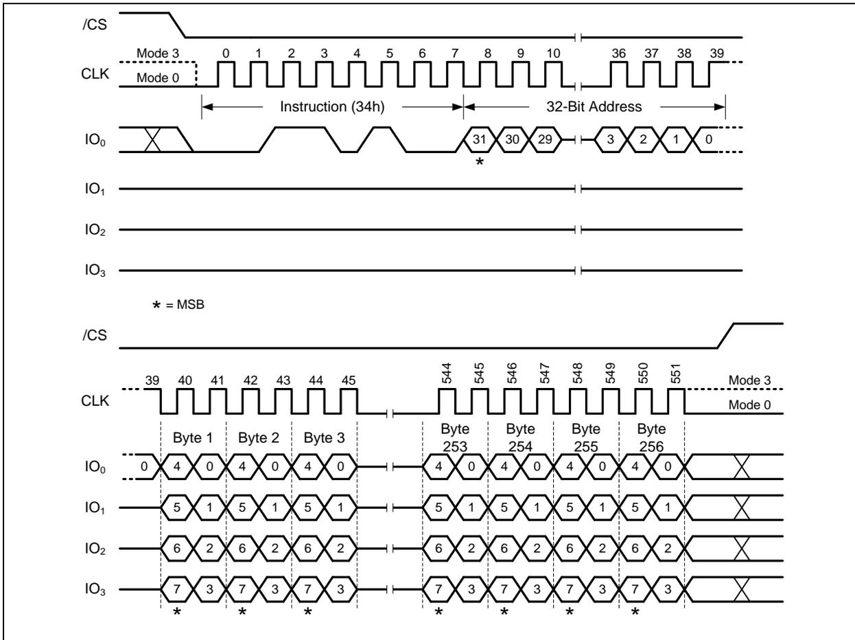
Figure 35. Quad Input Page Program with 4-Byte Addr.
