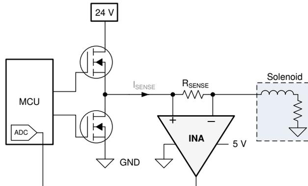
**Figure 8-2. Current Sensing in a Solenoid Application**
