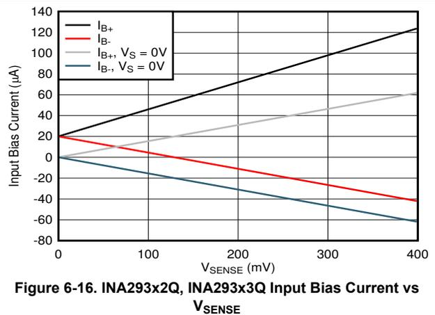
Figure 6-16. INA293x2Q, INA293x3Q Input Bias Current vs  $V_{\text{SENSE}}$
