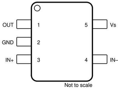
**Figure 5-1. INA293A-Q1: DBV Package 5-Pin SOT-23 Top View**
