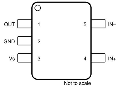
**Figure 5-2. INA293B-Q1: DBV Package 5-Pin SOT-23 Top View**
