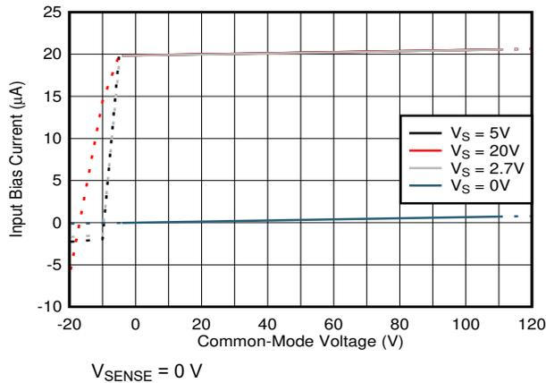
Figure 6-13. Input Bias Current vs Common-Mode Voltage
