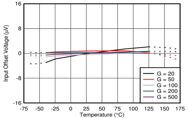
Figure 6-6. Input Offset Voltage vs Temperature
