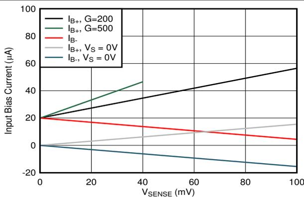
Figure 6-17. INA293x4Q, INA293x5Q Input Bias Current vs  $V_{\text{SENSE}}$
