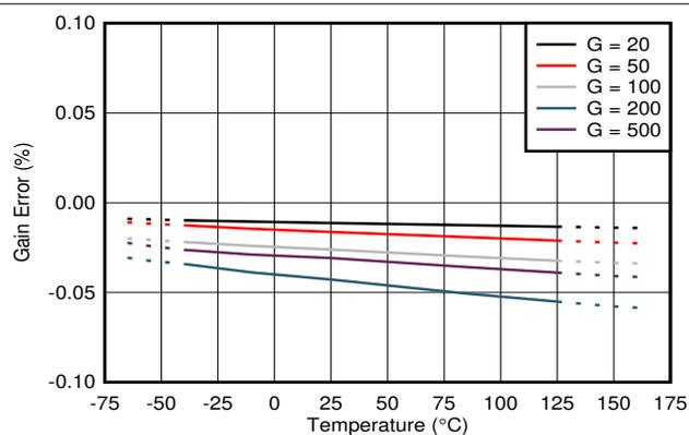
Figure 6-10. Gain Error vs Temperature
