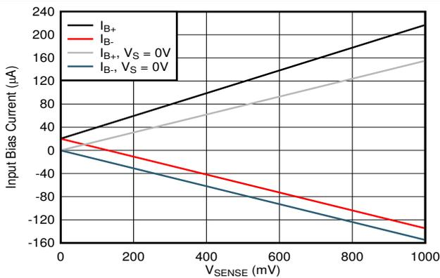
Figure 6-15. INA293x1Q Input Bias Current vs  $V_{\text{SENSE}}$
