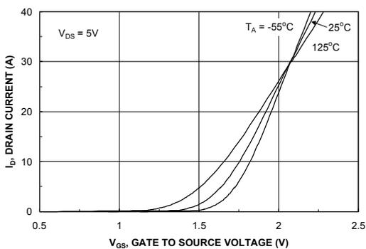
Figure 5. Transfer Characteristics.
