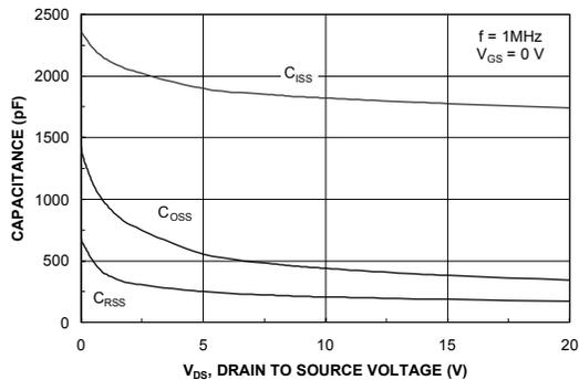
Figure 8. Capacitance Characteristics.
