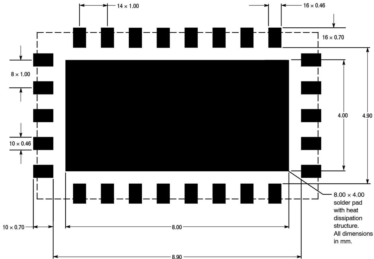
Figure 3. PCB Pad Layout for 10 mm × 6 mm Module
