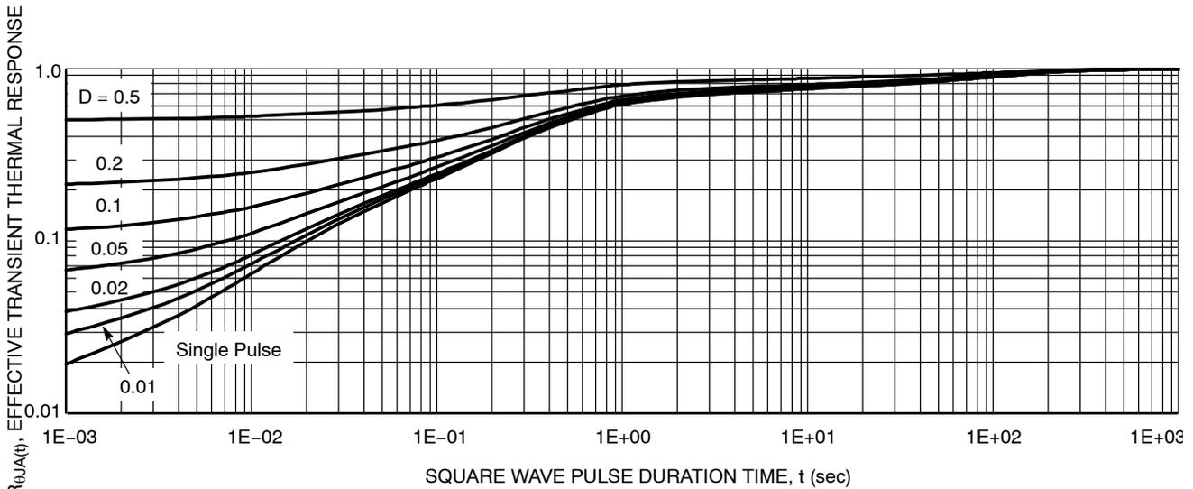
**Figure 11. FET Thermal Response Normalized to R<sub>θJA</sub> at Steady State (1 inch Pad)**
