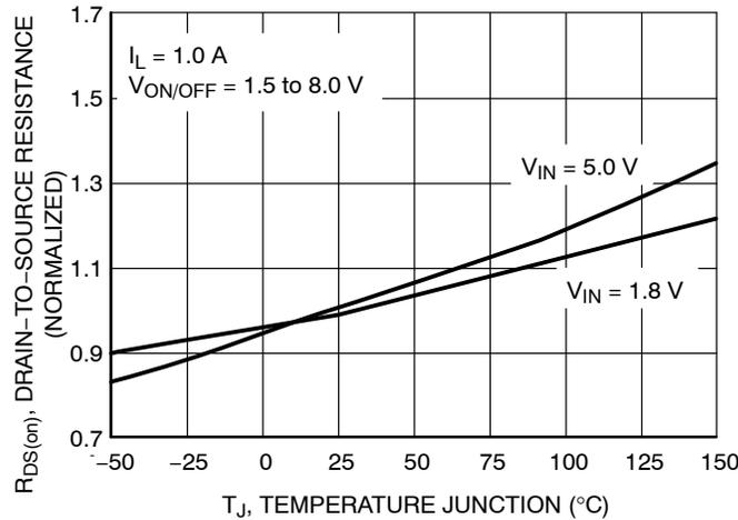
Figure 6. Normalized On Resistance Variation with Temperature
