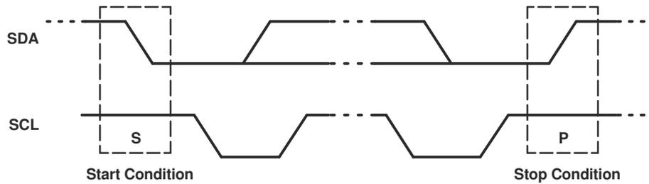
**Figure 8-3. Definition Of Start And Stop Conditions**
