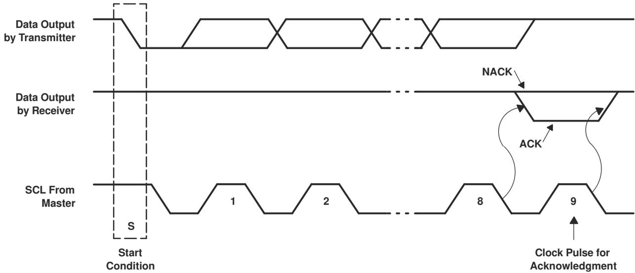
Figure 8-5. Acknowledgment On I<sup>2</sup>C Bus
