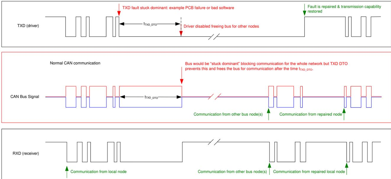
**Figure 8-4. Example Timing Diagram for TXD Dominant Timeout**
