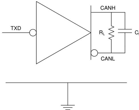
**Figure 7-1. I<sub>CC</sub> Test Circuit**
