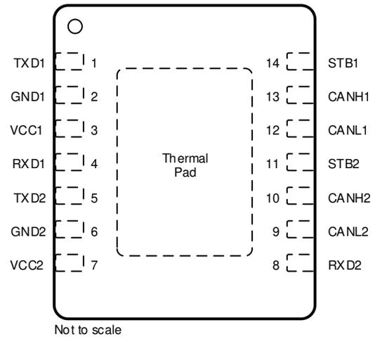
**Figure 5-2. DMT Package TCAN1046-Q1, 14 Pin VSON, Top View**
