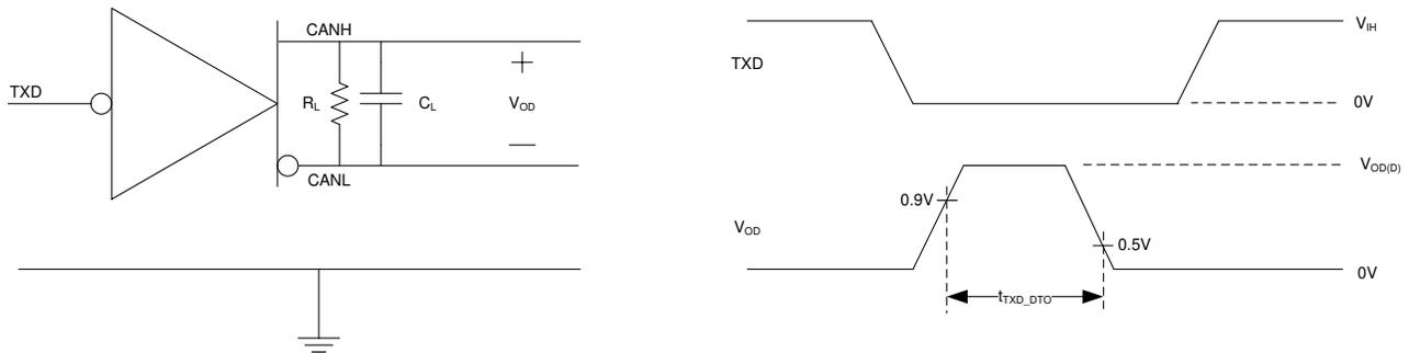
**Figure 7-6. TXD Dominant Timeout Test Circuit and Measurement**
