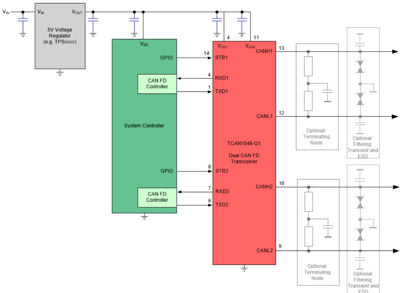
Figure 9-1. Transceiver Application Using 5 V I/O Connections
