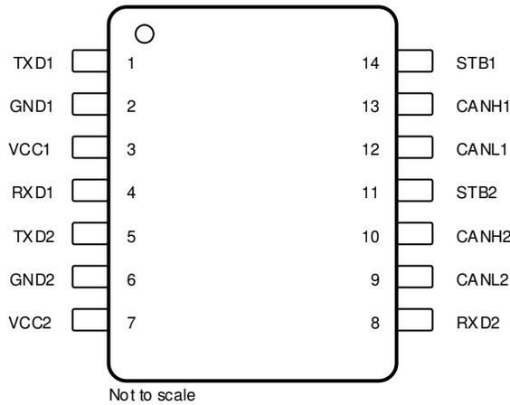
**Figure 5-1. D Package TCAN1046-Q1, 14 Pin SOIC, Top View**
