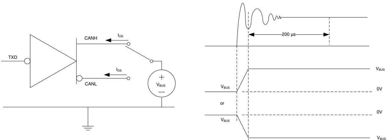
**Figure 7-7. Driver Short-Circuit Current Test and Measurement**
