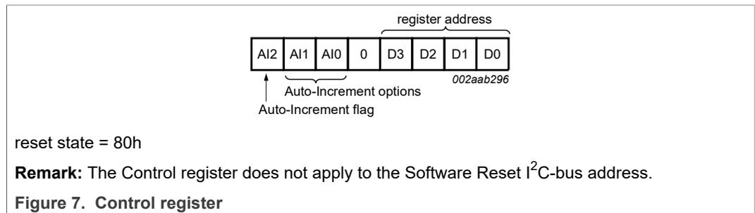
**Remark:** The Control register does not apply to the Software Reset I<sup>2</sup>C-bus address.
