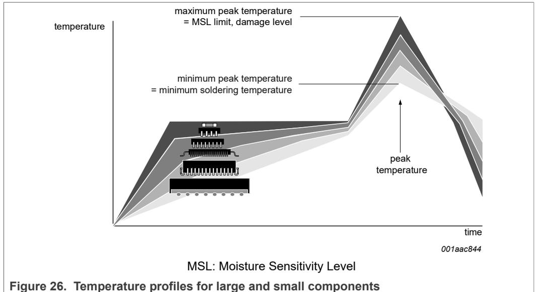
Figure 26. Temperature profiles for large and small components
