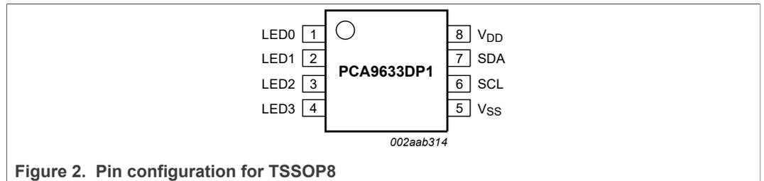
Figure 2. Pin configuration for TSSOP8
