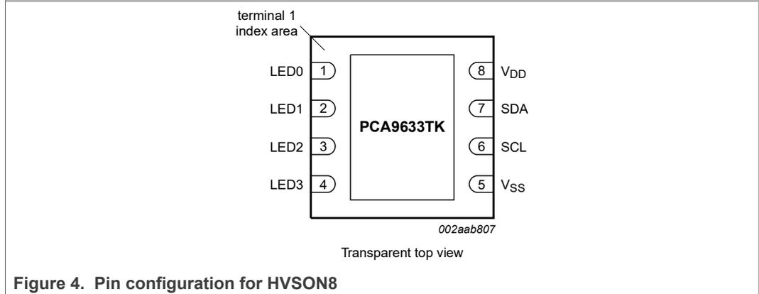
Figure 4. Pin configuration for HVSON8
