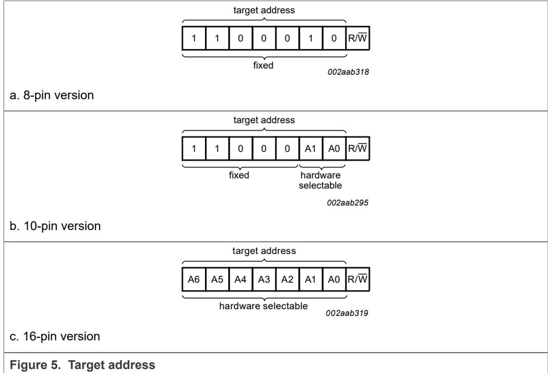
The last bit of the address byte defines the operation to be performed. When set to logic 1 a read is selected, while a logic 0 selects a write operation.
