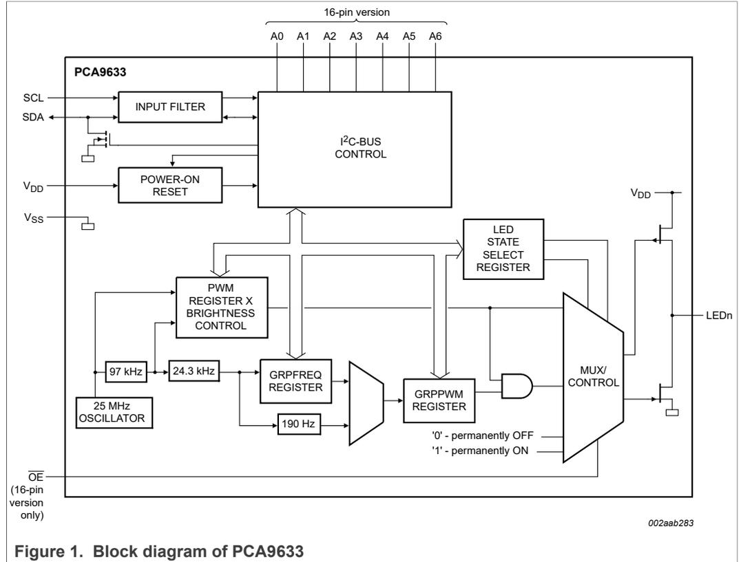
Figure 1. Block diagram of PCA9633
