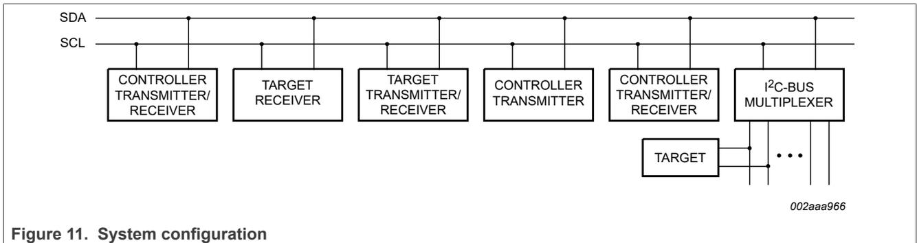
Figure 11. System configuration
