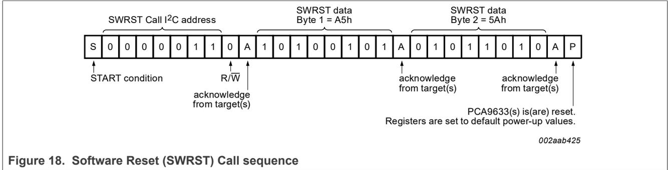
Figure 18. Software Reset (SWRST) Call sequence
