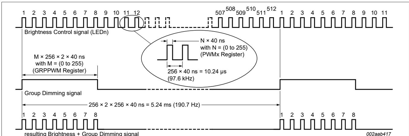
Minimum pulse width for LEDn Brightness Control is 40 ns.
