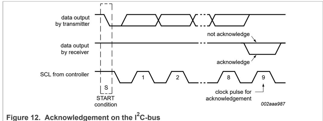
Figure 12. Acknowledgement on the I<sup>2</sup>C-bus
