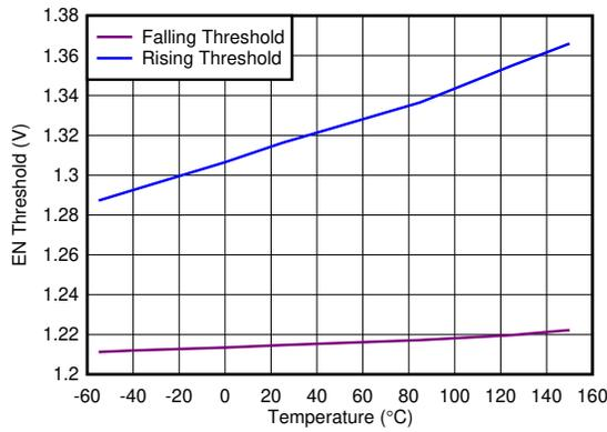
**Figure 6-27. EN Threshold vs Temperature**
