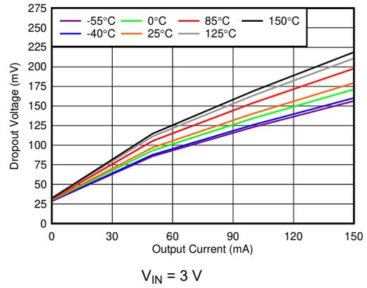
Figure 6-8. Dropout Voltage ( $V_{Do}$ ) vs  $I_{OUT}$
