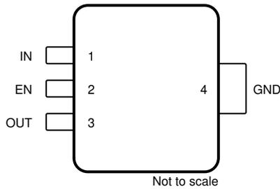
**Figure 5-1. DCY Package, 4-Pin SOT-223, Top View**
