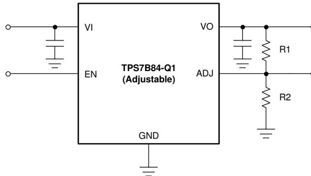
Figure 8-7. Typical Application Schematic for the TPS7B84-Q1
