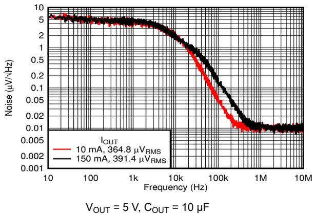
Figure 6-12. Noise vs Frequency at 5.0 V
