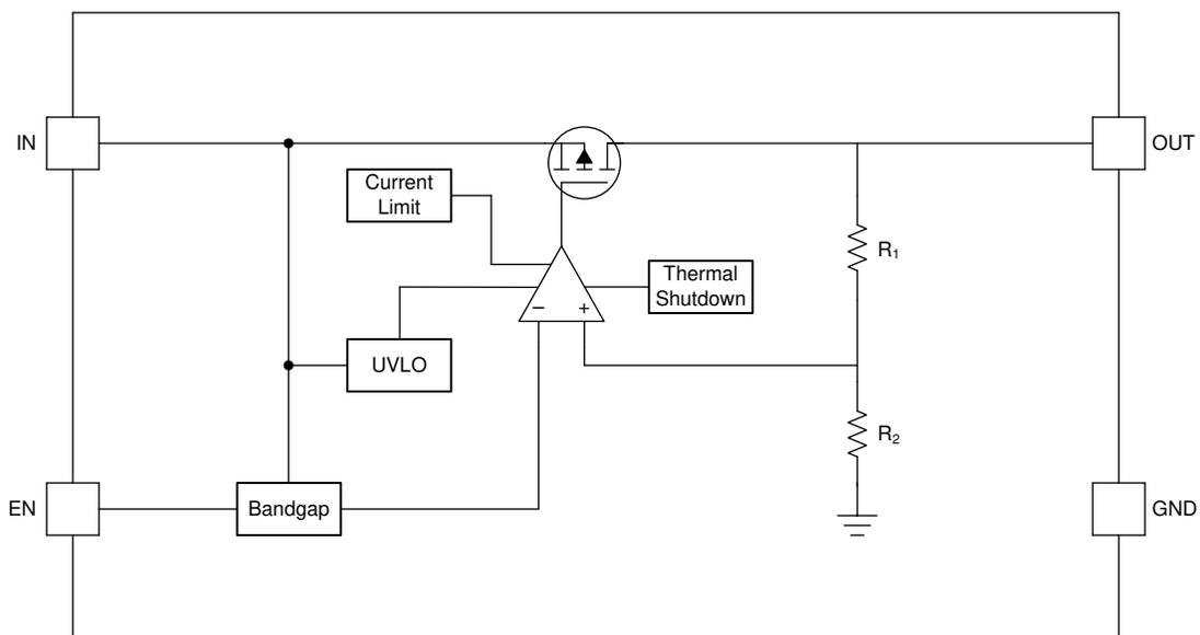
**Figure 7-2. Fixed Output Block Diagram**
