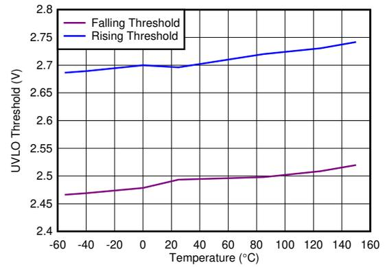
**Figure 6-28. Undervoltage Lockout (UVLO) Threshold vs Temperature**
