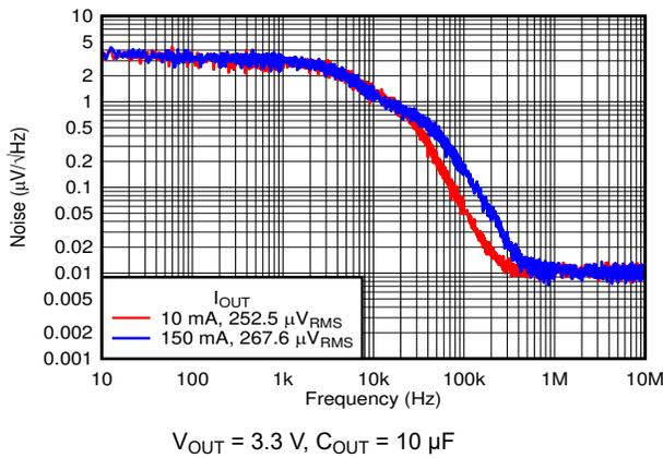
Figure 6-11. Noise vs Frequency at 3.3 V
