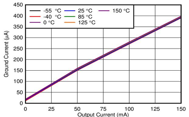
**Figure 6-24. Ground Current ( $I_{GND}$ ) vs  $I_{OUT}$**
