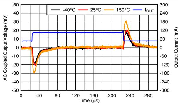
$V_{OUT} = 5\ \text{V}$ ,  $I_{OUT} = 45\ \text{mA}$  to  $105\ \text{mA}$ , slew rate =  $0.1\ \text{A}/\mu\text{s}$ ,
