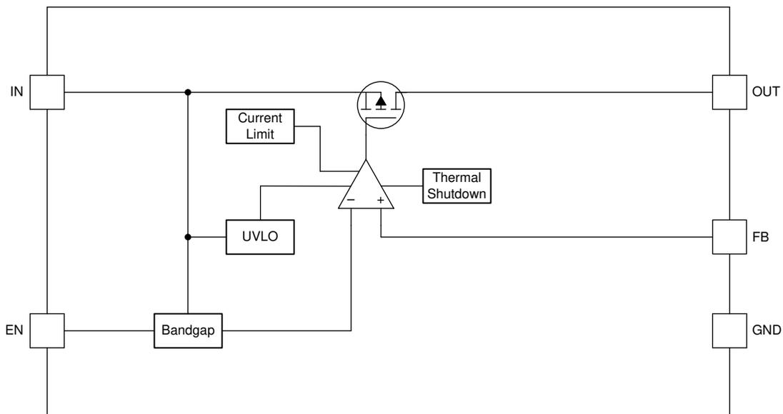
**Figure 7-1. Adjustable Output Block Diagram**
