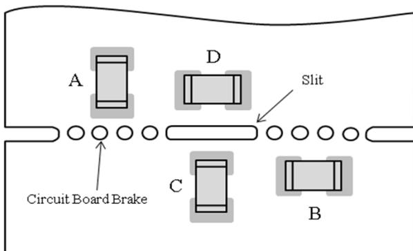
Stress strength according to the mounting position:
