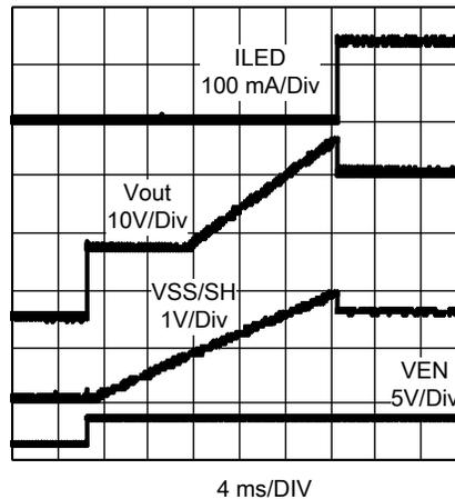
Figure 15. Typical Startup Waveforms (From power-on, DIM = high)
