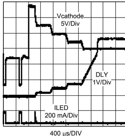
Figure 26. LED String Short Fault and UVP Detection
