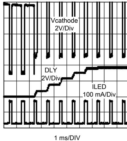
Figure 24. DLY Charging, 1 LED Open Fault
