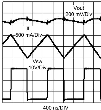
Figure 17. Inductor Current, SW Voltage, and V<sub>OUT</sub>
