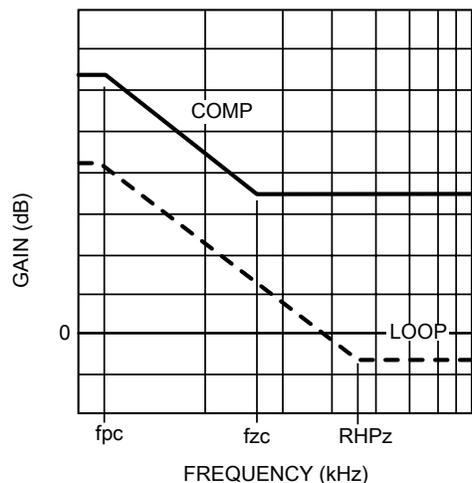
**Figure 20. Typical Compensation and Total Loop Bode Plots**
