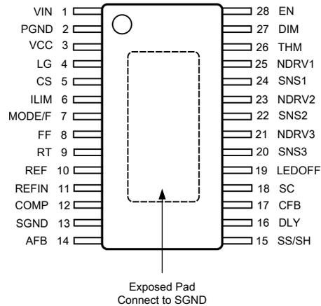
**Figure 1. 28 Lead Plastic Exposed Pad TSSOP
