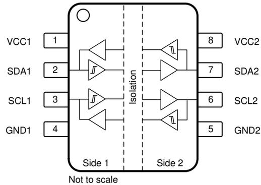
**Figure 5-1. ISO1540-Q1 D Package 8-Pin SOIC Top View**
