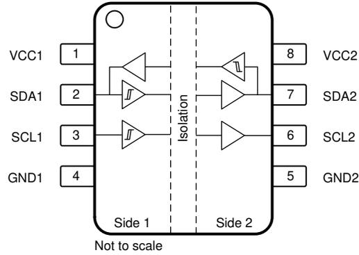
**Figure 5-2. ISO1541-Q1 D Package 8-Pin SOIC Top View**
