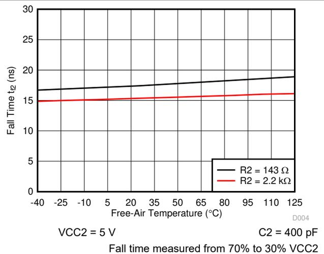
**Figure 6-7. Side 2: Output Fall Time vs Free-Air Temperature**
