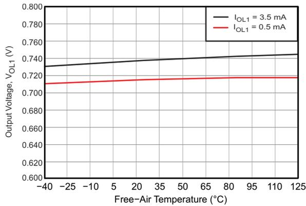
**Figure 6-2. Side 1: Output Low Voltage vs Free-Air Temperature**
