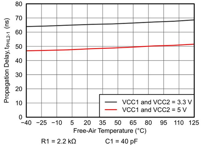
Figure 6-15.  $t_{PHL2-1}$  Propagation Delay vs Free-Air Temperature
