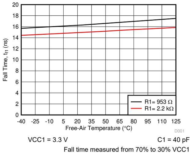
**Figure 6-4. Side 1: Output Fall Time vs Free-Air Temperature**
