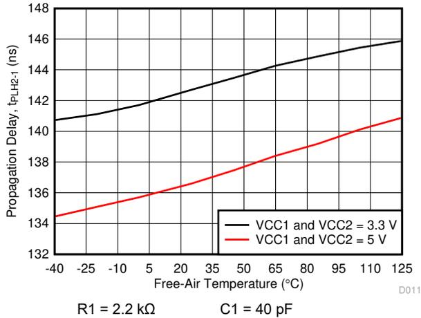
Figure 6-14.  $t_{PLH2-1}$  Propagation Delay vs Free-Air Temperature
