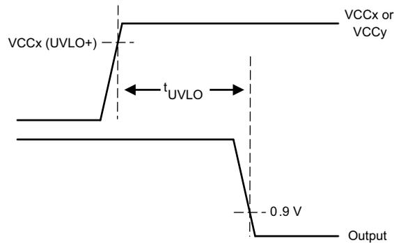
**Figure 7-4.  $t_{UVLO}$  Test Circuit and Timing Diagrams**
