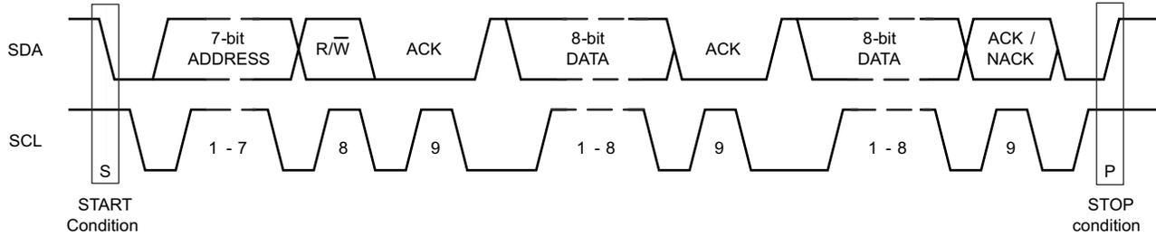
**Figure 8-2. Timing Diagram of a Complete Data Transfer**
