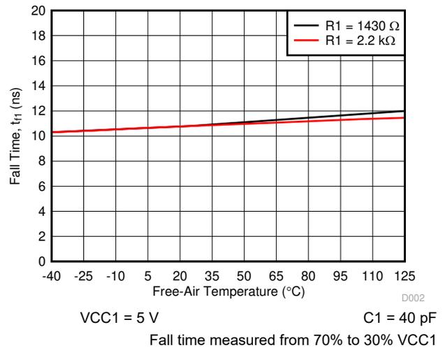
**Figure 6-5. Side 1: Output Fall Time vs Free-air Temperature**
