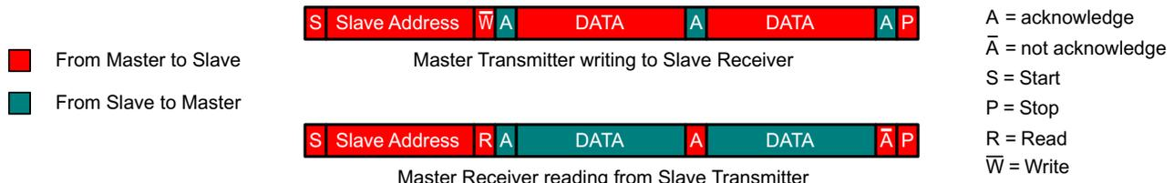
**Figure 8-3. Transmit or Receive Mode Changes During a Data Transfer**
