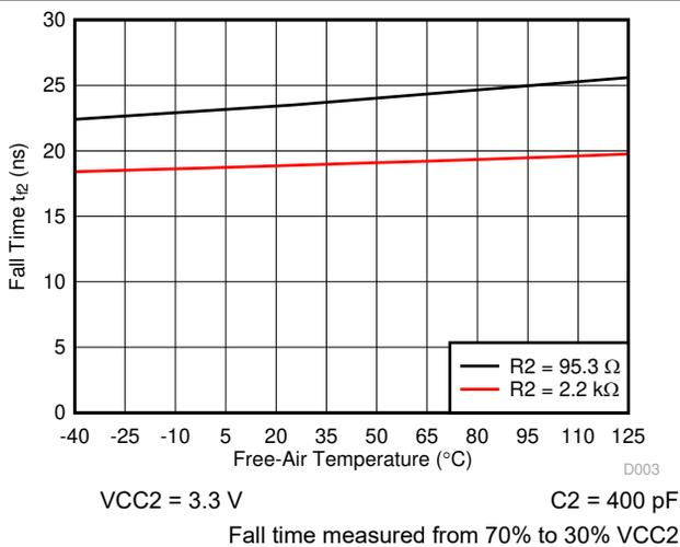
**Figure 6-6. Side 2: Output Fall Time vs Free-Air Temperature**
