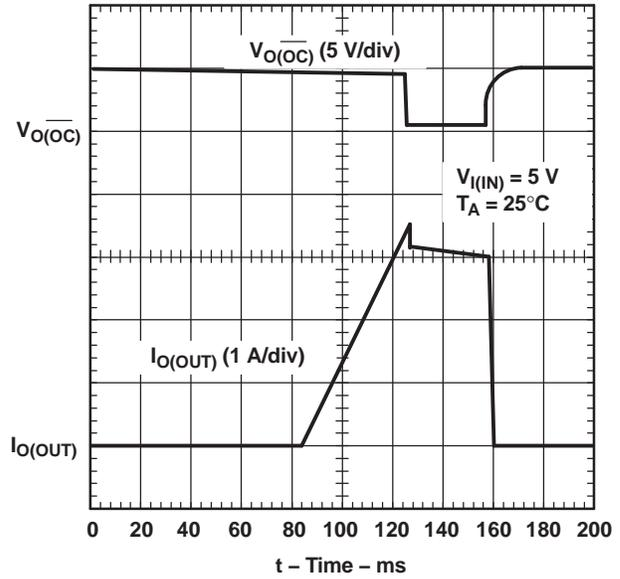
Figure 11. TPS2034, Ramped Load on Enabled Device
