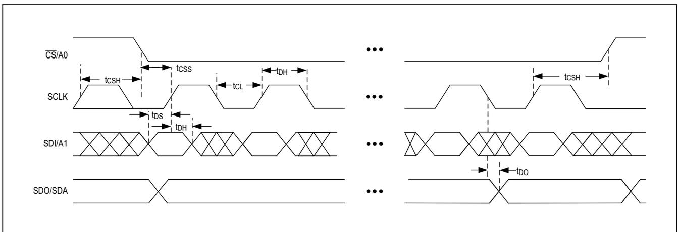
Figure 6. SPI Timing
