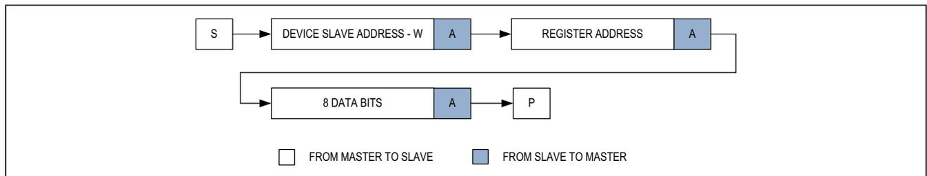
Figure 11. I<sup>2</sup>C Byte Write
