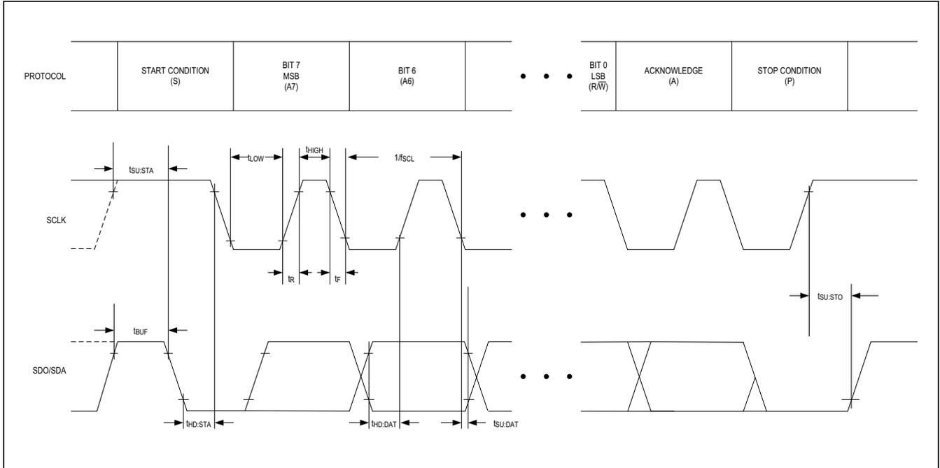
Figure 7. I<sup>2</sup>C Timing
