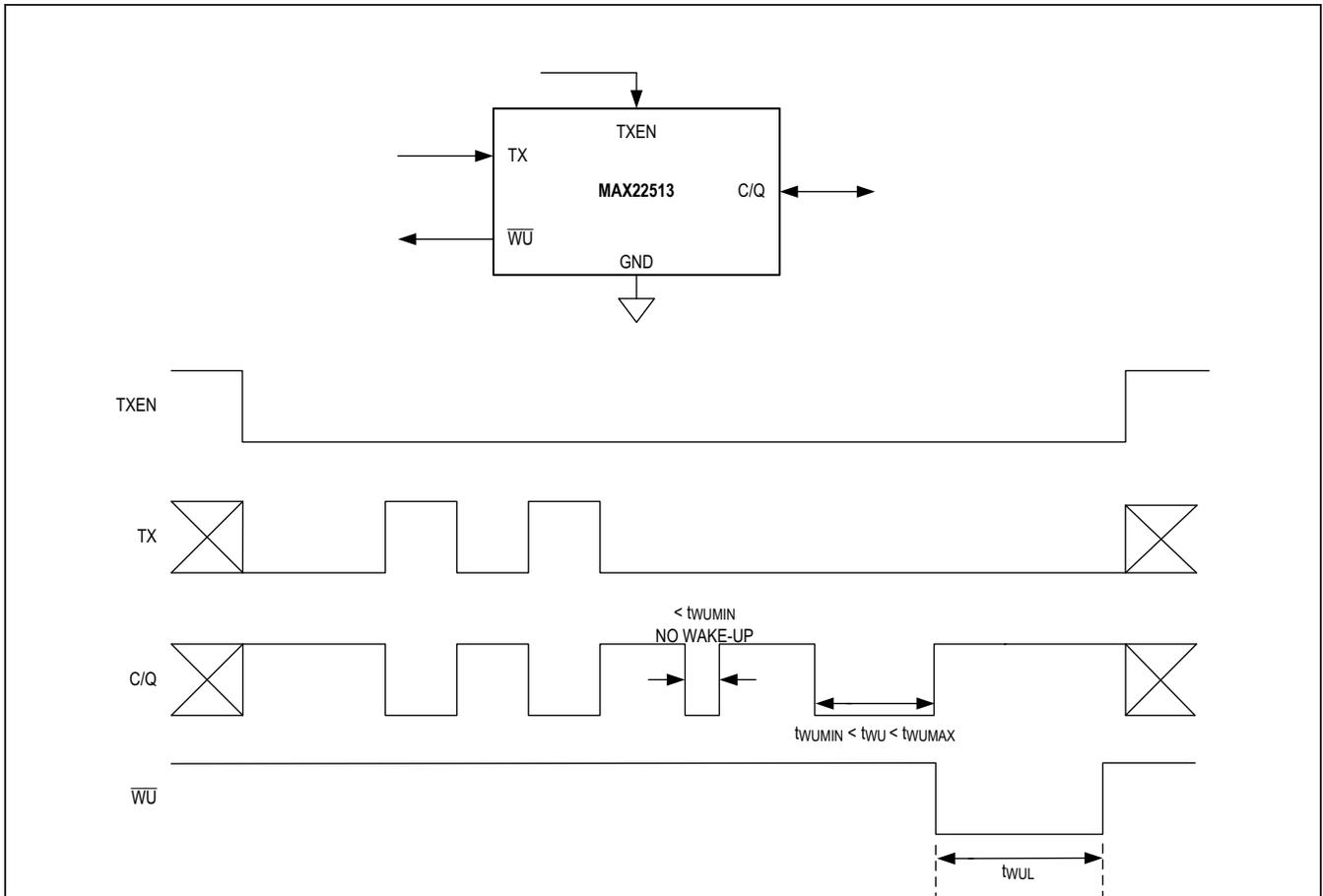
Figure 5. Wake-Up Timing
