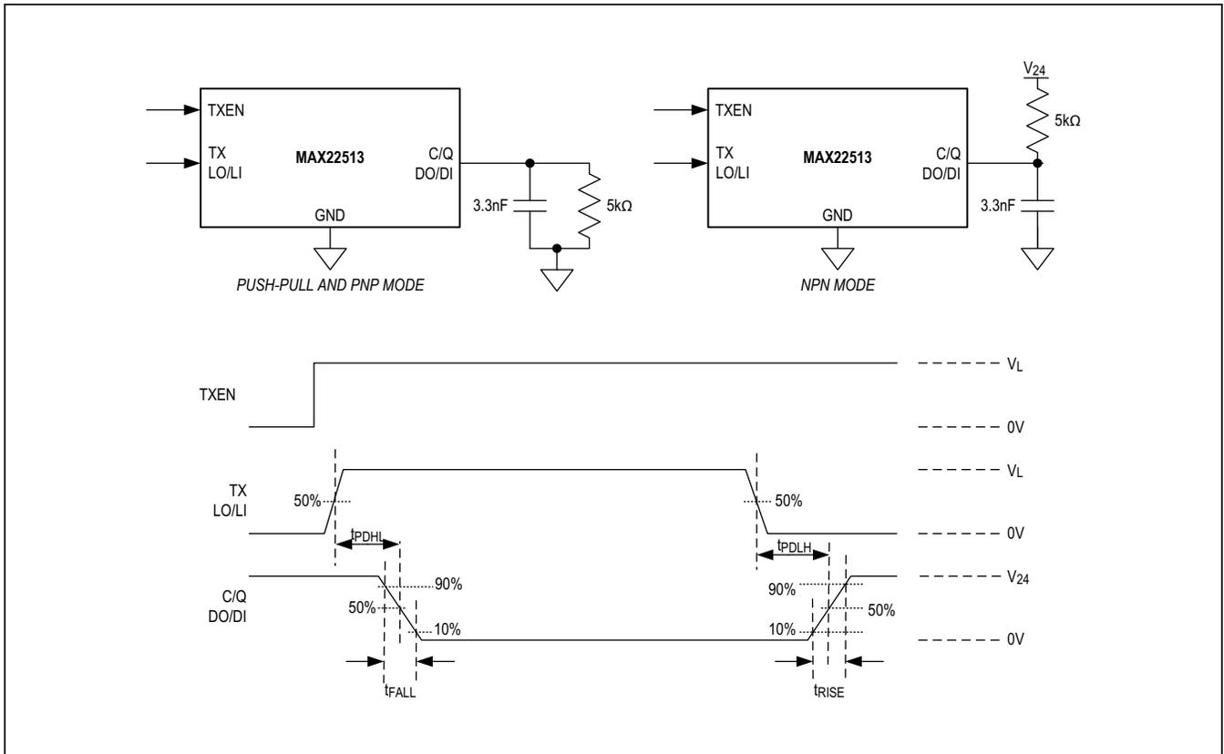
Figure 1. C/Q and DO/DI Driver Propagation Delays
