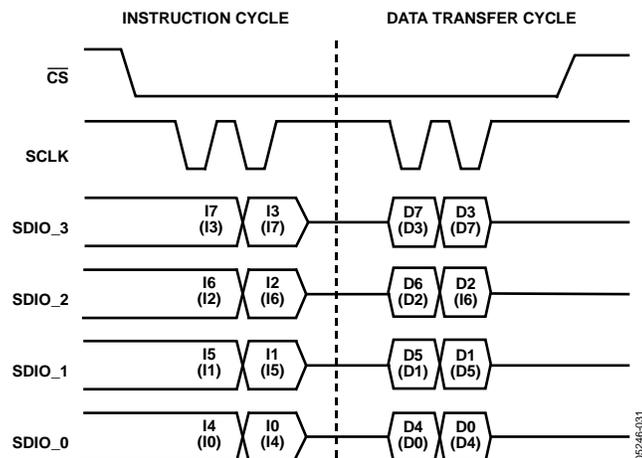
Figure 49. 4-Bit Serial Mode Read Timing—Clock Stall High
