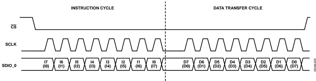
Figure 43. Single-Bit Serial Mode Write Timing—Clock Stall Low
