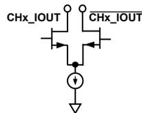
TERMINATE OUTPUTS INTO AVDD. DO NOT EXCEED VOLTAGE COMPLIANCE OF OUTPUTS.
