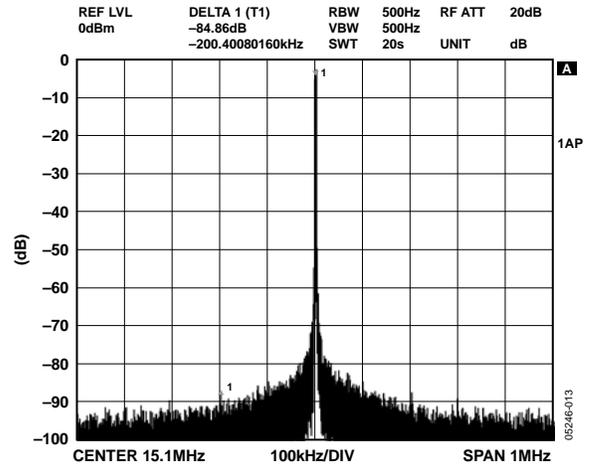
Figure 13. NBSFDR,  $\pm 1$  MHz,  $f_{OUT} = 15.1$  MHz,  $f_{CLK} = 500$  MSPS
