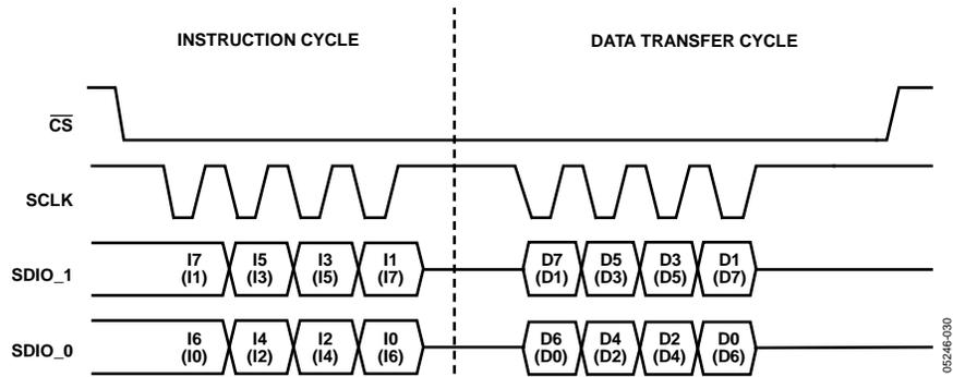
Figure 48. 2-Bit Serial Mode Read Timing—Clock Stall High
