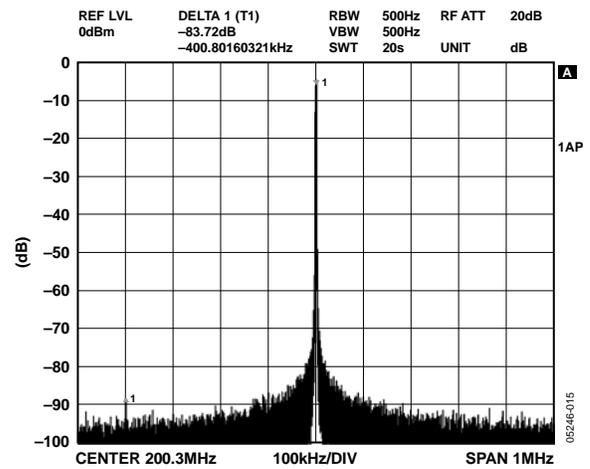
Figure 15. NBSFDR,  $\pm 1$  MHz,  $f_{OUT} = 200.3$  MHz,  $f_{CLK} = 500$  MSPS
