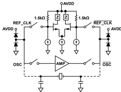
REF\_CLK INPUTS ARE INTERNALLY BIASED AND NEED TO BE AC-COUPLED. OSC INPUTS ARE DC-COUPLED.
