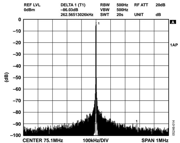
Figure 14. NBSFDR,  $\pm 1$  MHz,  $f_{OUT} = 75.1$  MHz,  $f_{CLK} = 500$  MSPS
