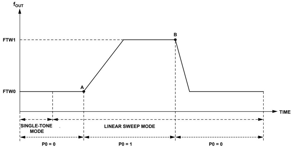
AT POINT A: LOAD RISING RAMP RATE REGISTER, APPLY RDW<31:0>
