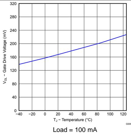
Figure 19. Gate Drive Low Voltage vs Temperature
