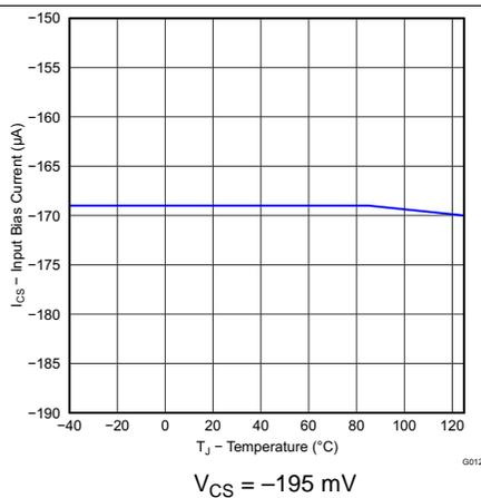
Figure 23. Current Sense Input Bias Current vs Temperature
