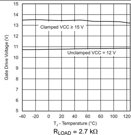
Figure 18. Gate Drive High Voltage vs Temperature
