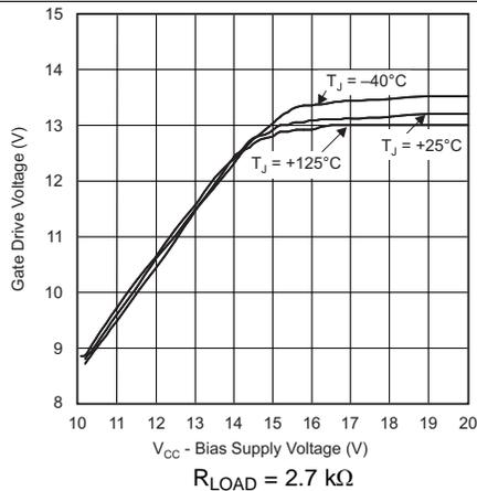
Figure 17. Gate Drive Output High vs VCC
