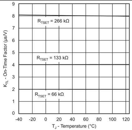
Figure 10. On-Time Factor Phase A and B vs Temperature
