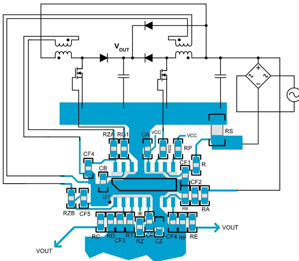
PHB and VREF pins are connected by a jumper on the back of the board.
