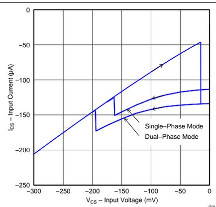
Figure 24. Current Sense Input Bias Current vs Input Voltage
