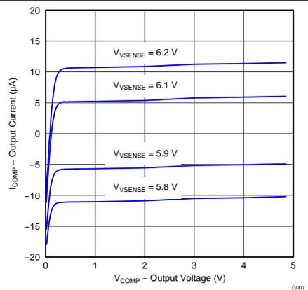
Figure 8. Error Amplifier Output Current vs Output Voltage
