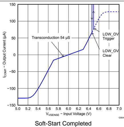
Figure 5. Error Amplifier Output Current vs Input Voltage
