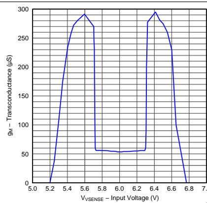
Figure 6. Error Amplifier Transconductance vs VSENSE
