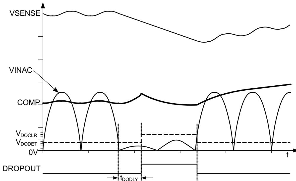
**Figure 32. AC-Line Dropout Timing With Illustrative System Behavior**
