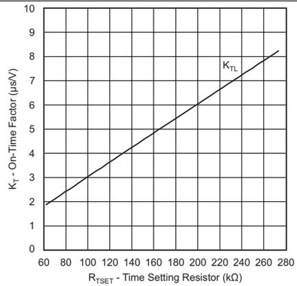
Figure 9. On-Time Factor vs Time Setting Resistor
