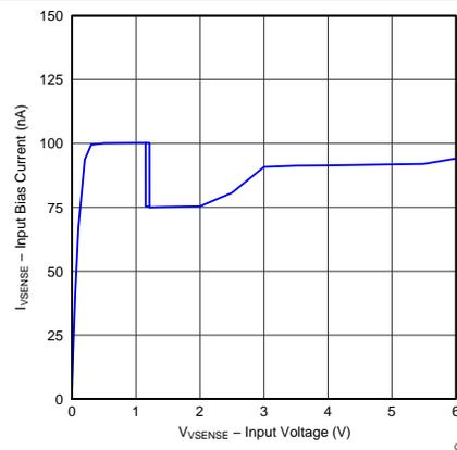
Figure 4. VSENSE Input Bias Current vs Input Voltage
