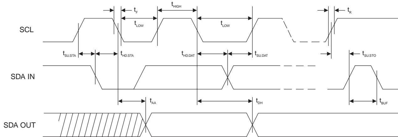
**Figure 5-2. Write Cycle Timing**
