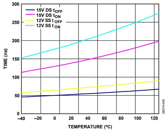
Figure 14.  $t_{ON}/t_{OFF}$  vs. Temperature
