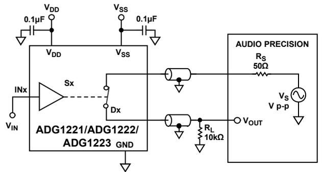
Figure 32. Test Circuit 10—Total Harmonic Distortion + Noise
