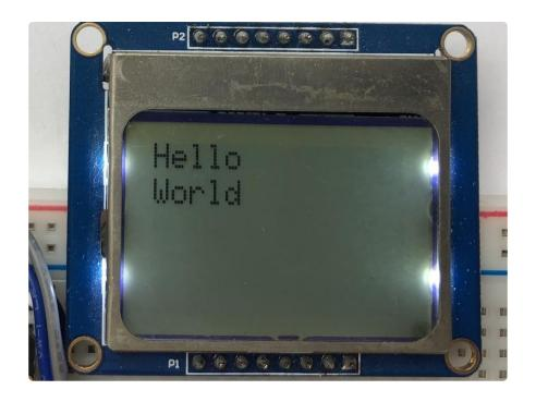
That's all there is to drawing on the Nokia 5110/3310 LCD display with CircuitPython! The drawing functions are basic but provide building blocks for more advanced usage. For example you can display text with sensor readings or other state, or even program a simple game like pong!
