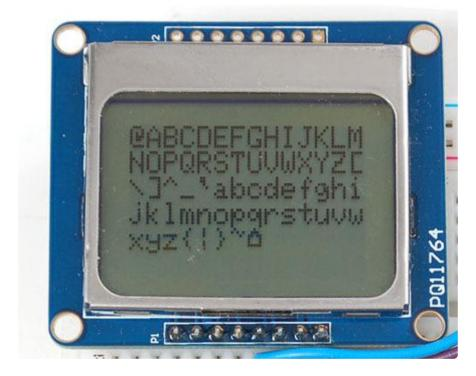
This is a quick tutorial for our 84x48 pixel monochrome LCD display. These displays are small, only about 1.5" diameter, but very readable due and comes with a backlight. This display is made of 84x48 individual pixels, so you can use it for graphics, text or bitmaps. These displays are inexpensive, easy to use, require only a few digital I/O pins and are fairly low power as well.
