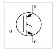
600V  $I_{C(nom)} = 8.0A$   $V_{CE(on)} typ. = 1.55V @ 8.0A$   $@ T_{C} = 25^{\circ}C$ Motor Control IGBT
