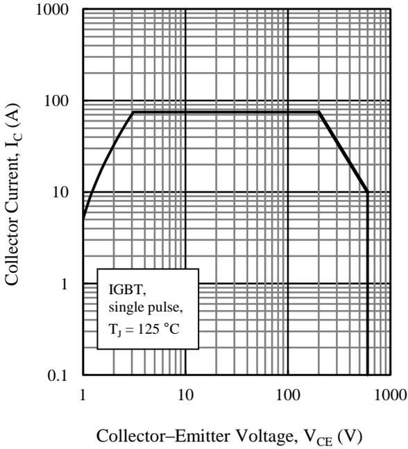
Figure 2. IGBT Reverse Bias Safe Operating Area
