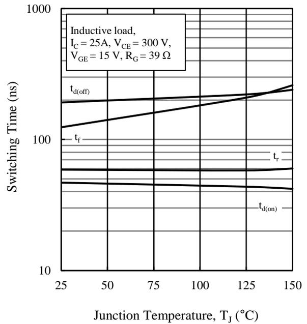
Figure 13. Switching Time vs. Junction Temperature
