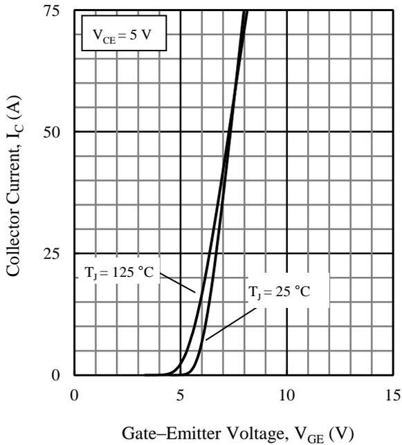
Figure 8. Transfer Characteristics
