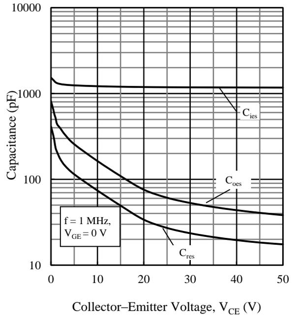
Figure 11. Capacitance Characteristics
