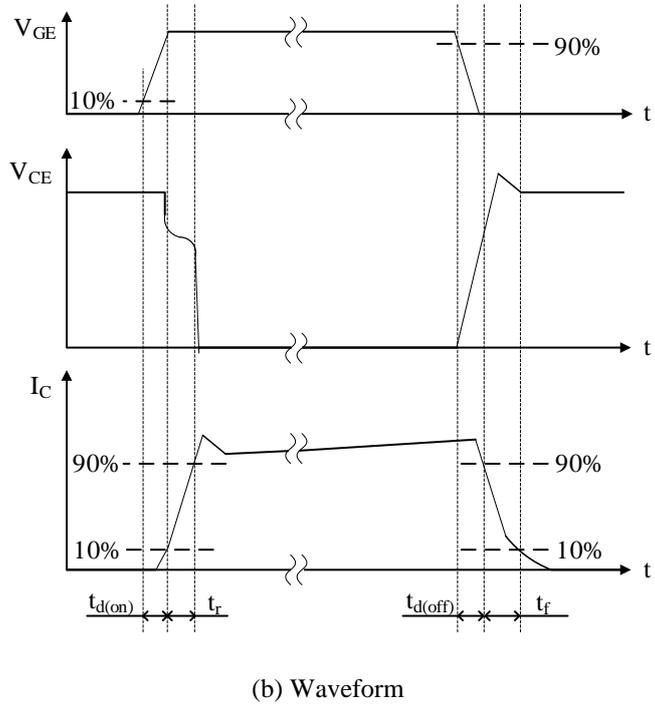
Figure 1. Test Circuits and Waveforms of  $dv/dt$  and Switching Time
