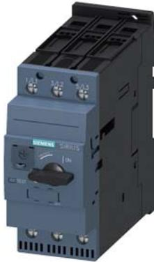
Circuit breaker size S2 for motor protection, CLASS 10 A-release 70...80 A N-release 1040 A screw terminal increased switching capacity
