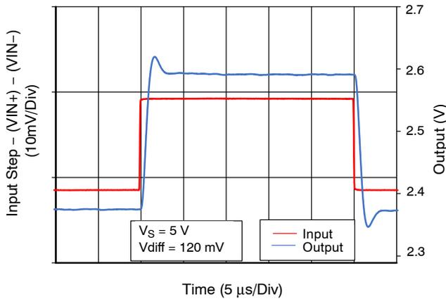
**Figure 21b. Small Signal Step Response Non-Inverting, G20**
