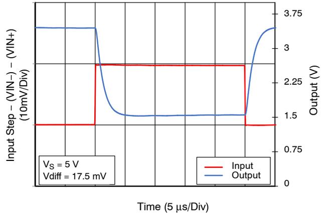
**Figure 21c. Small Signal Step Response Inverting, G200**
