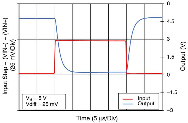
**Figure 22c. Small Signal Step Response Inverting, G200**
