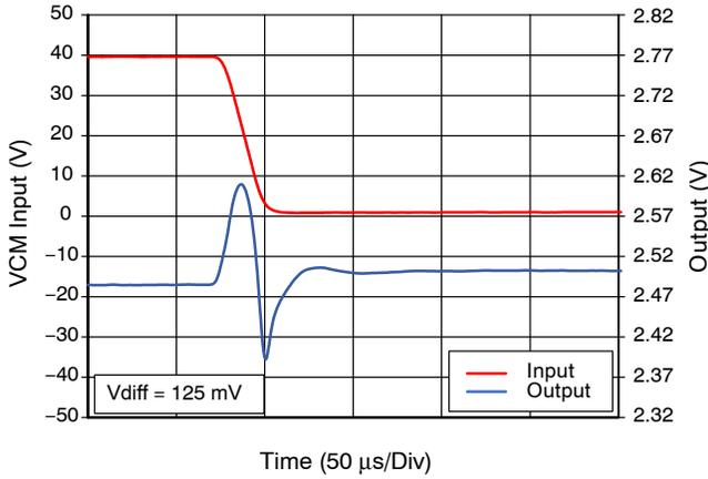
**Figure 23b. Common Mode Step Response Falling, G20**
