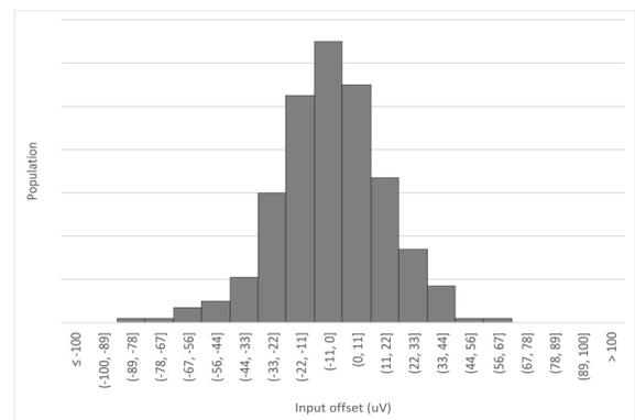
**Figure 3d. Input Offset Voltage Distribution, G200**
