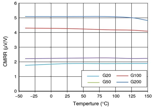
**Figure 6. Common Mode Rejection Ratio vs Temperature**
