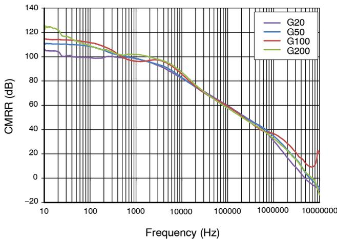
**Figure 10. Common Mode Rejection Ratio vs Frequency**
