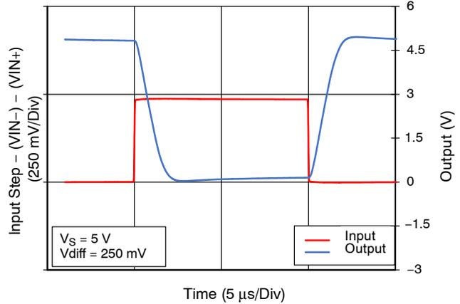
**Figure 22a. Large Signal Step Response Inverting, G20**
