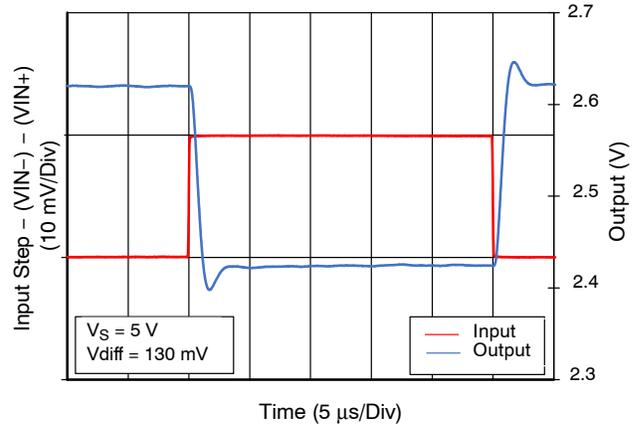
**Figure 21a. Small Signal Step Response Inverting, G20**
