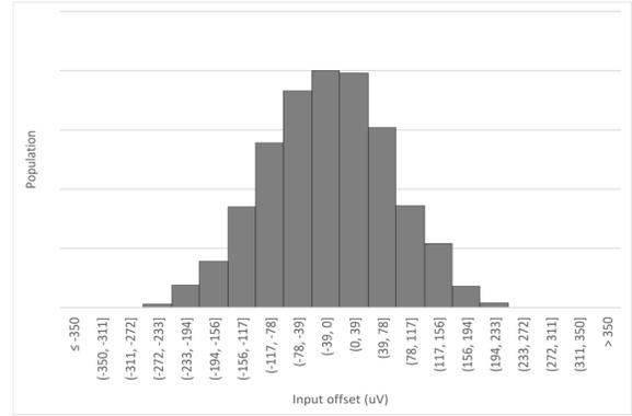
**Figure 3b. Input Offset Voltage Distribution, G50**
