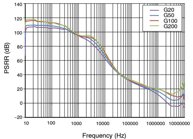
**Figure 11. Power Supply Rejection Ratio vs Frequency**
