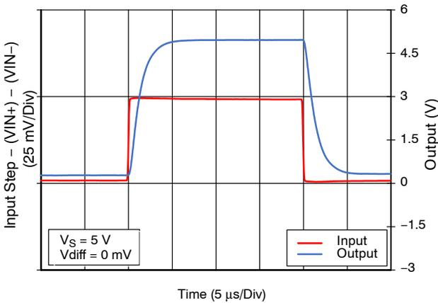
**Figure 22b. Large Signal Step Response Non-Inverting, G20**
