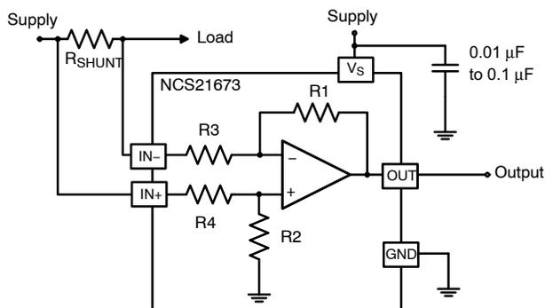
Figure 1. Example Application Schematic of High-Side Current Sensing
