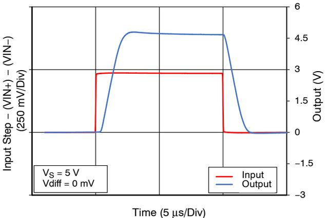
**Figure 22d. Large Signal Step Response Non-Inverting, G200**
