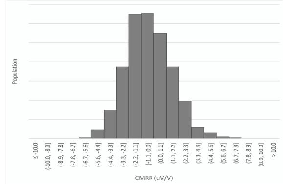
**Figure 5c. Common Mode Rejection Ratio Distribution, G100**
