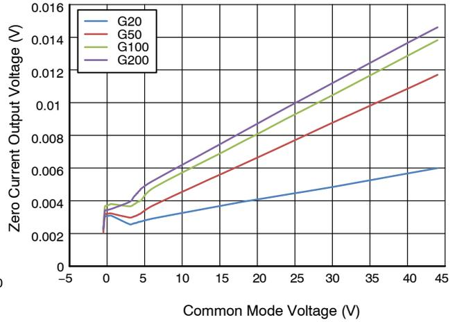
**Figure 9. Zero Current Output vs Common Mode Voltage**
