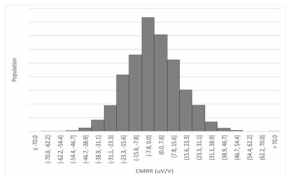
**Figure 5a. Common Mode Rejection Ratio Distribution, G20**
