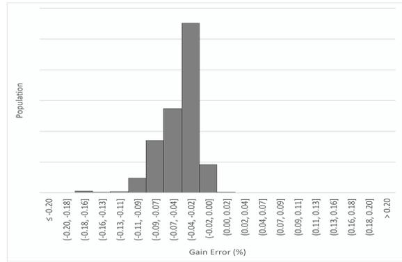
**Figure 7d. Gain Error Distribution, G200**
