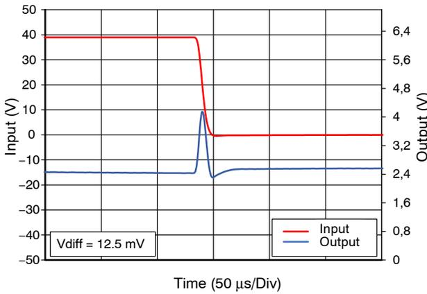
**Figure 23d. Common Mode Step Response Rising, G200**
