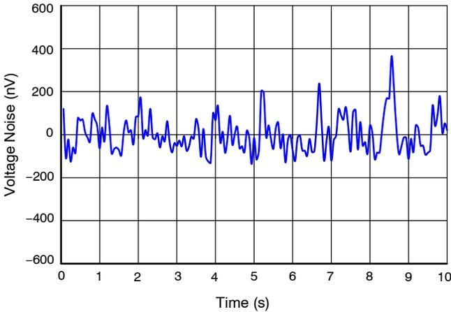
**Figure 20. 0.1-Hz to 10-Hz Voltage Noise (Referred-To-Input)**
