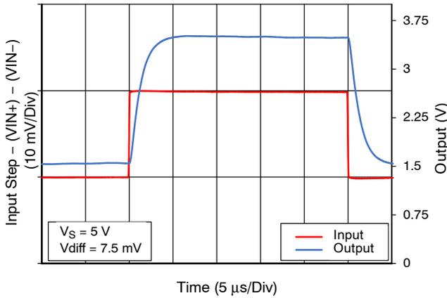
**Figure 21d. Small Signal Step Response Non-Inverting, G20**
