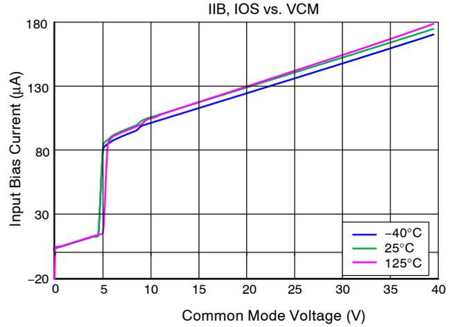
**Figure 15. Input Bias Current vs Common Mode Voltage**
