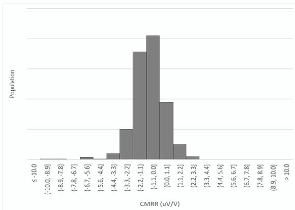
**Figure 5d. Common Mode Rejection Ratio Distribution, G200**
