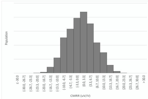
**Figure 5b. Common Mode Rejection Ratio Distribution, G50**
