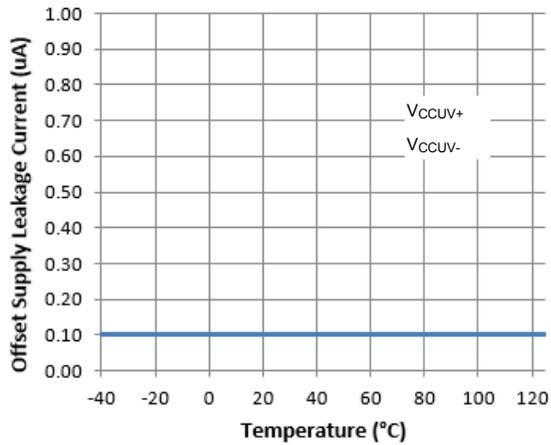
Figure 25. Offset Supply Leakage Current vs. Temperature
