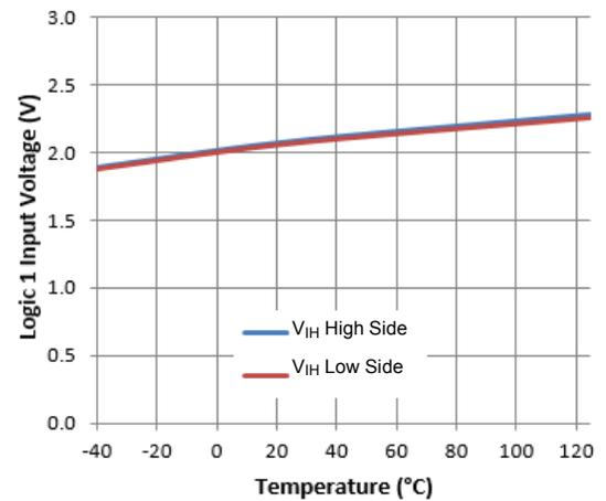
Figure 22. Logic 1 Input Voltage vs. Temperature
