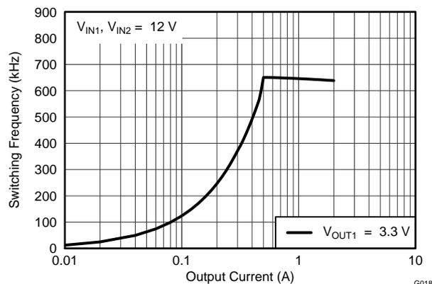
Figure 18. VO1 = 3.3V, SW-frequency vs Output Current (PWP)
