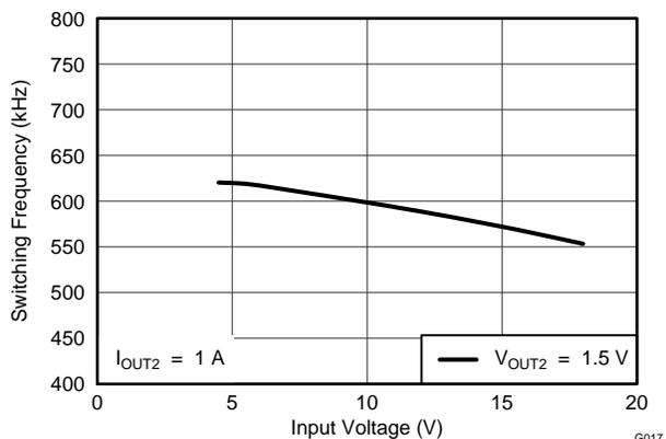
Figure 17. VO2 = 1.5V, SW-frequency vs Input Voltage (PWP)
