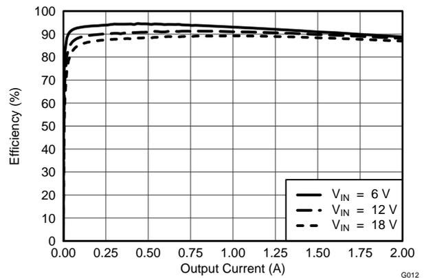
Figure 12. VO1 = 3.3V, Efficiency vs Output Current
