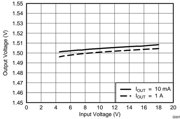
Figure 7. VO2 = 1.5V Output Voltage vs Input Voltage
