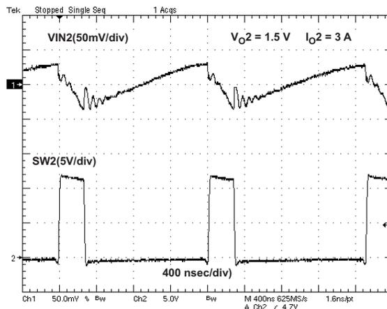
Figure 23.  $VIN2$  Input Voltage Ripple ( $I_{O2} = 3\text{ A}$ )
