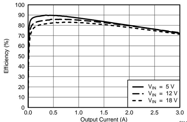
Figure 14. VO2 = 1.5V, Efficiency vs Output Current
