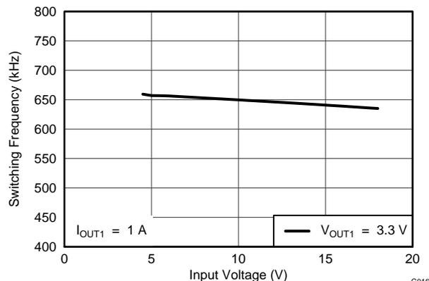
Figure 16. VO1 = 3.3V, SW-frequency vs Input Voltage (PWP)
