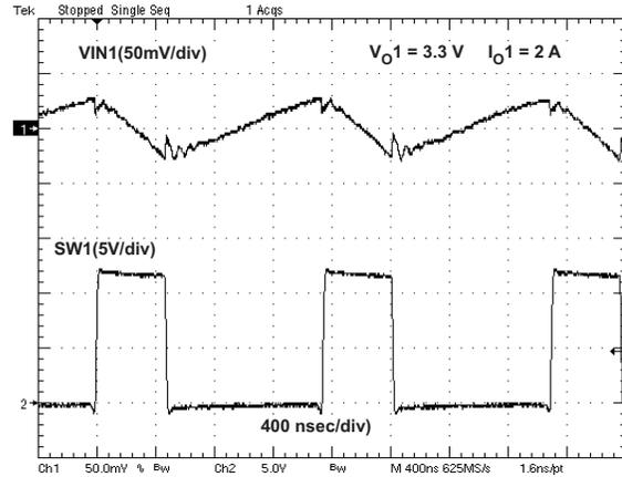
Figure 22.  $VIN1$  Input Voltage Ripple ( $I_{O1} = 2\text{ A}$ )
