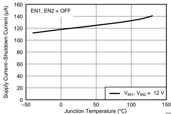
Figure 2. Input Shutdown Current vs Junction Temperature
