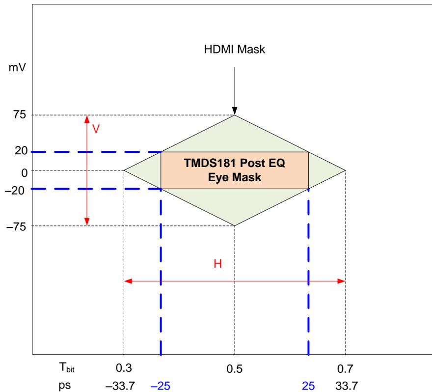
Figure 13. Input Eye Mask Post EQ – TTP2\_EQ
