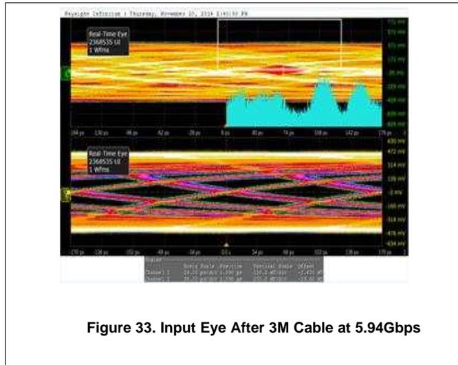
Figure 33. Input Eye After 3M Cable at 5.94Gbps
