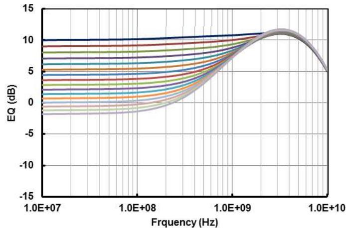
**Figure 27. Adaptive EQ Gain Curve for >3.4 Gbps**
