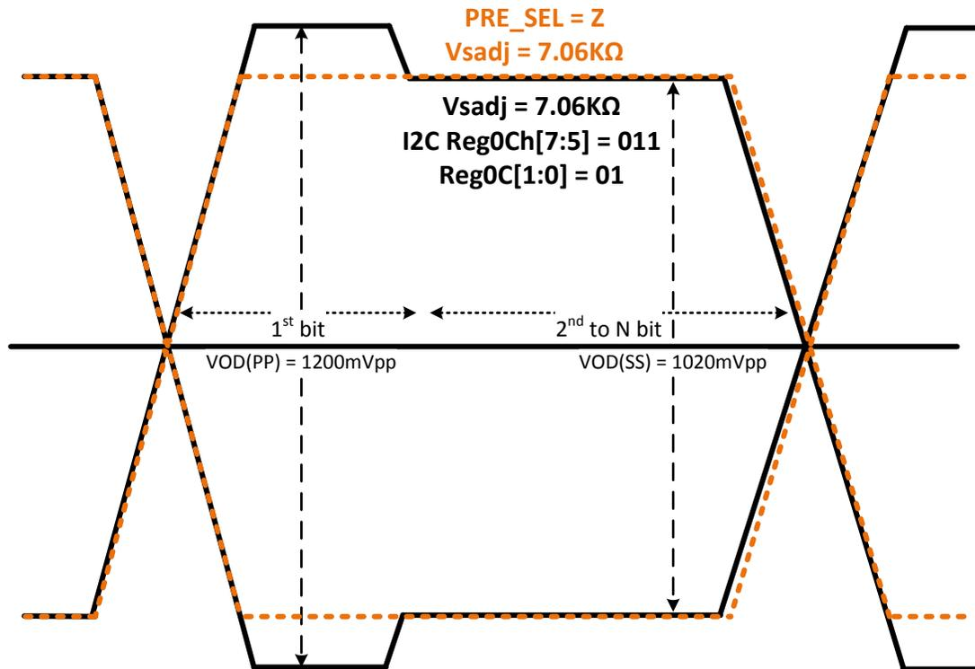
Figure 30. Output Pre-Emphasis Using I<sup>2</sup>C
