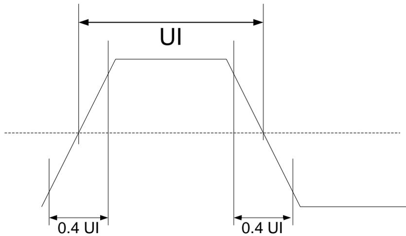
Figure 23. Rise and Fall Time of ARC
