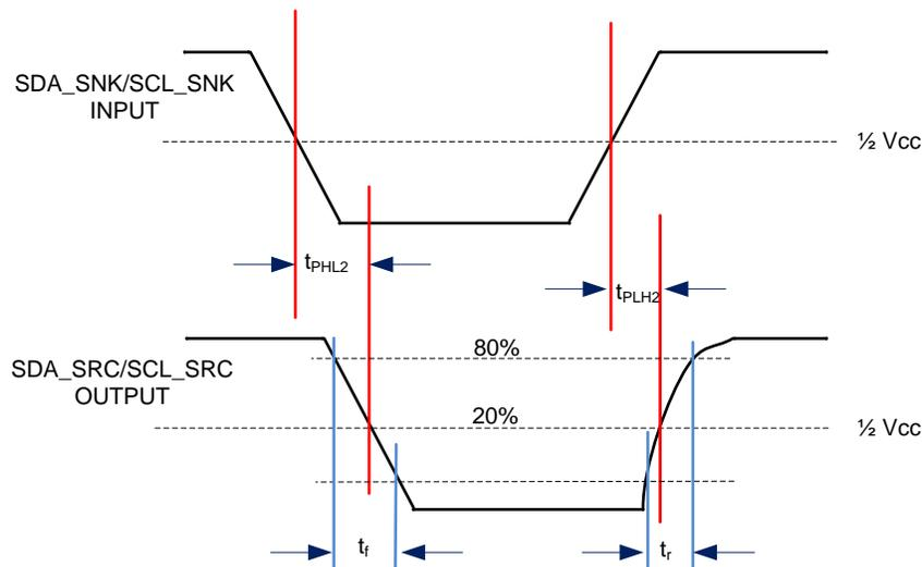
**Figure 21. DDC Propagation Delay – Sink to Source**
