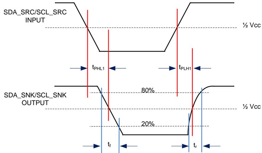
**Figure 20. DDC Propagation Delay – Source to Sink**
