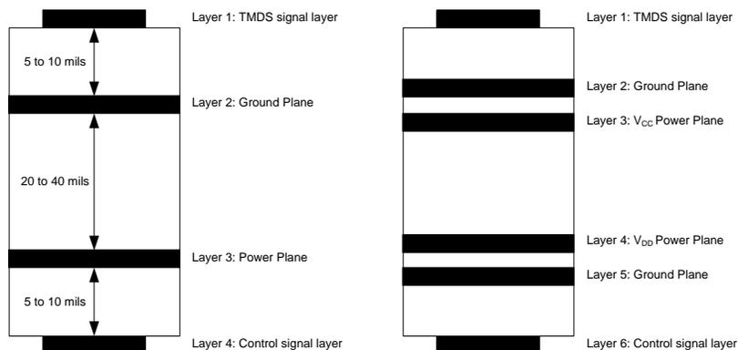
**Figure 38. Recommended 4- or 6-Layer PCB Stack**
