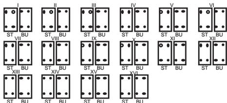
Figure 1: Coding for housings with one contact insert
